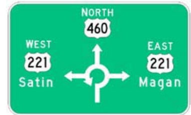
Figure 2. Diagrammatic roundabout guide sign.
