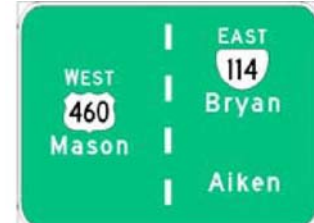
Figure 4. Vertical Lane line guide sign similar to those used at some New York roundabouts.
