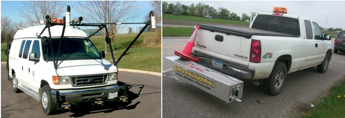
Figure 22. Examples of vehicles attached with profilometers for IRI assessments (from MnROAD 2008)
