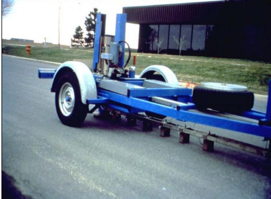
Figure 8. Falling weight deflectometer (FWD) machine (from Hall et al. 2001)
