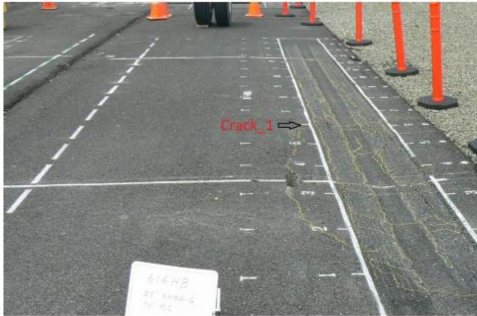
Figure 18. Structural failure of the underlying concrete layer appears as a crack in the AC overlay (from Rao et al. 2011)
