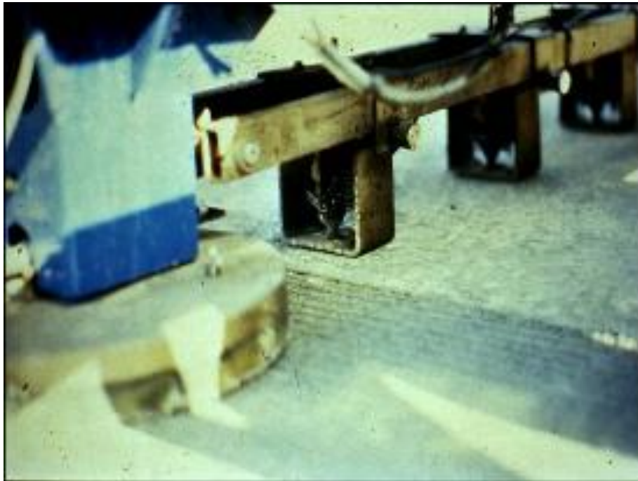
Figure 9. Close up of FWD load plate and deflection sensors (from Hall et al. 2001)
