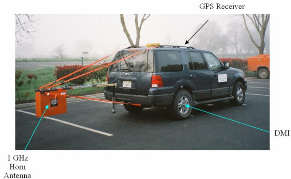
Figure 15. Vehicles equipped with ground penetrating radar (GPR) device (from Scullion 2006 (top) and Kohler et al. 2005 (bottom))
