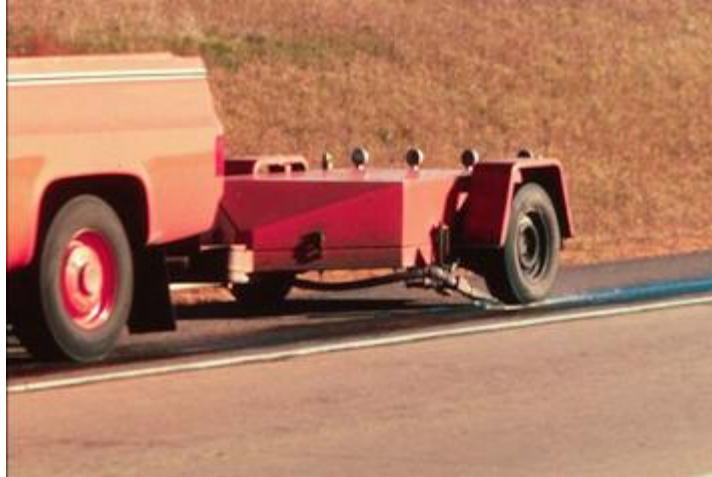
Figure 21. Friction testing trailer (from Hall et al. 2001)
