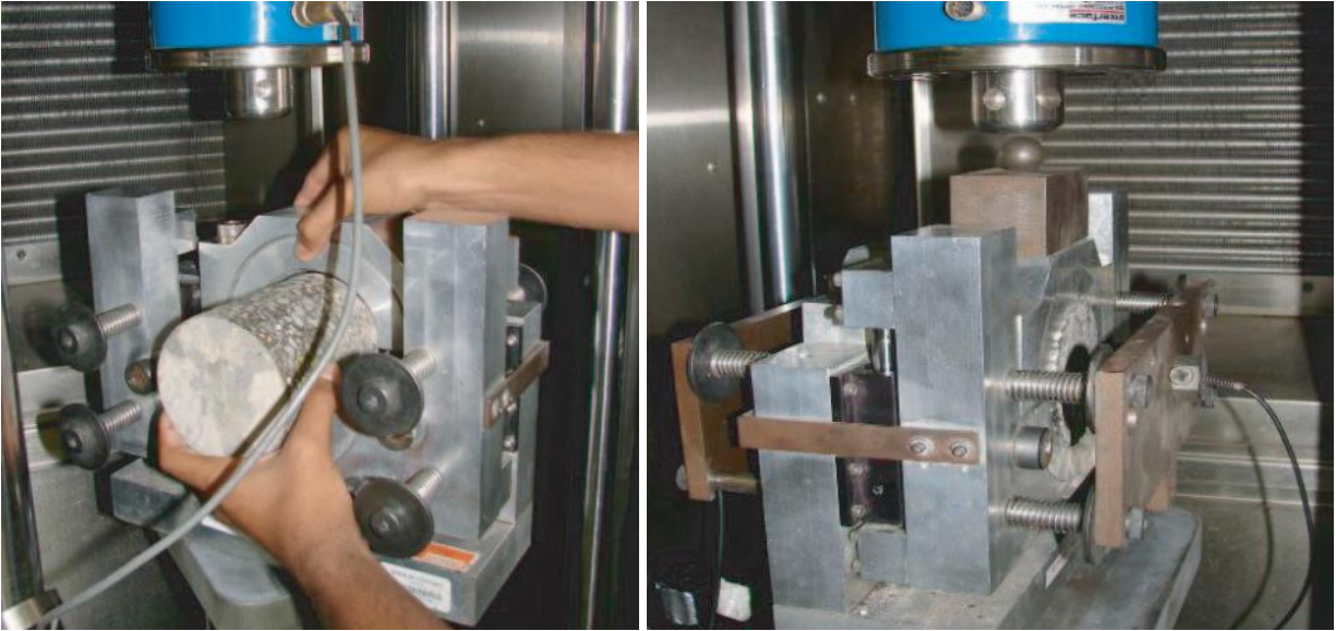
Figure 61. The Louisiana Interlayer Shear Strength Test (LISST) is an attachment to a standard load frame used to test the interlayer shear strength (From Mohammad et al. 2012)
