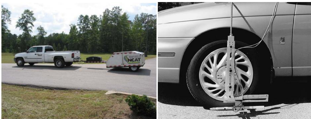
Figure 23. At left, trailer housing a microphone used to measure noise due to tire pavement interaction (from Hanson et al. 2004); at right, OBSI data collection using wheel-mounted probe (from Donovan and Lodico 2009)
