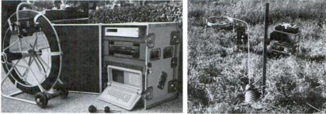
Figure 6. Video equipment for an advanced drainage survey (from Christopher and McGuffey 1997)
