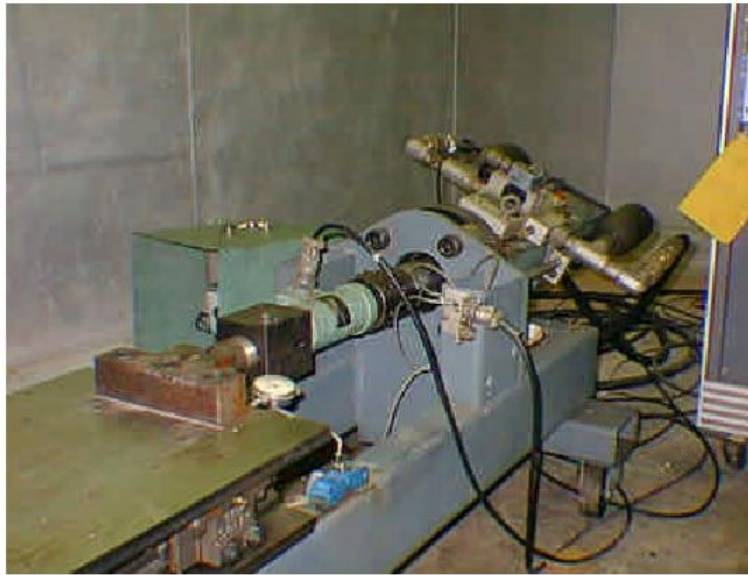
Figure 65. Texas Transportation Institute overlay tester (from Cleveland et al. 2002)
