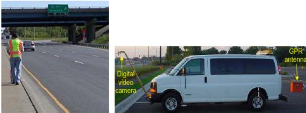
Figure 4. At left, inspector conducting a manual distress survey; at right, van outfitted to conducted a video distress survey (from Al-Qadi et al. 2009)
