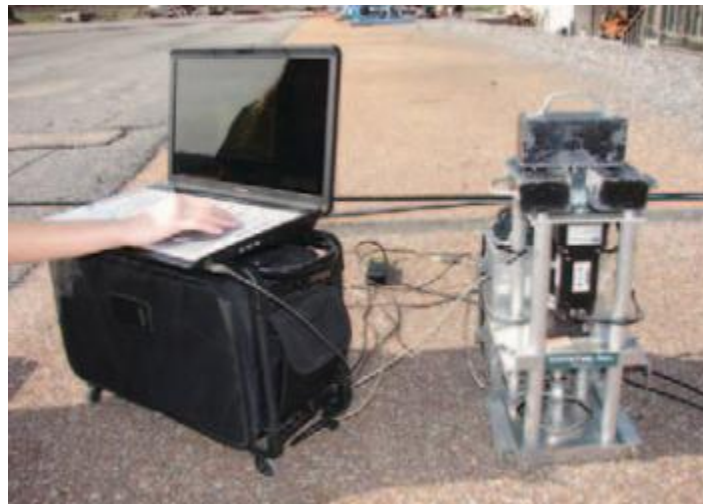
Figure 62. The Louisiana Tack Coat Quality Tester (LTCQT) is used to measure bond strength in the field (From Mohammad et al. 2012)
