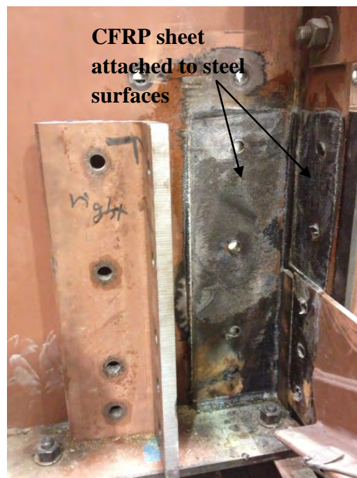
Figure 3.15: Trial 2: view of the interior face of the girder's web before application of the angles-with-plate-with-CFRP retrofit measure
