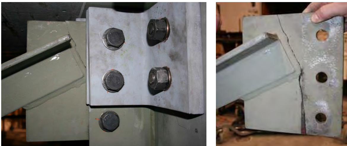
Figure 4.6: North cross frame failure during Trial 4N
