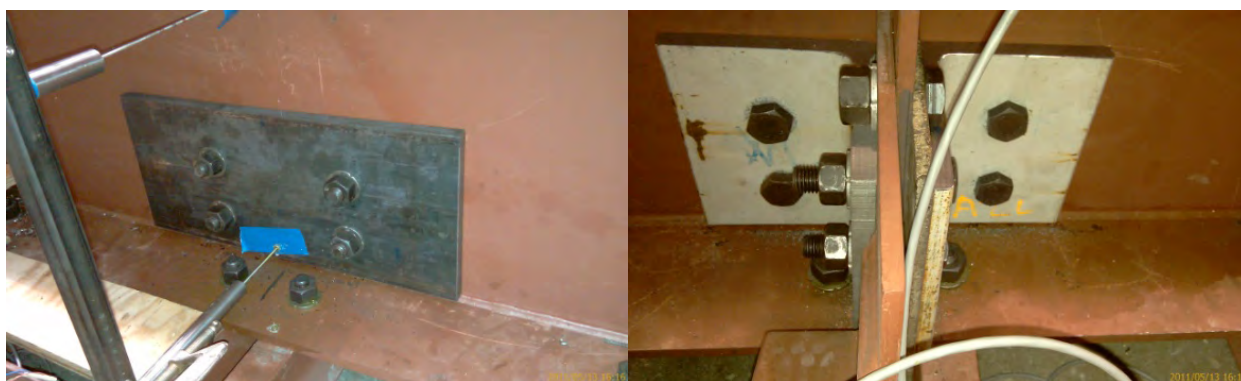
Figure 3.3: Angles-with-plate repair installed in the bottom web gap of the 2.8 m (9.3 ft) girder model
