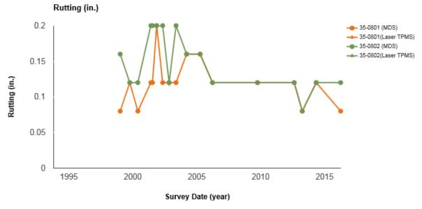
Figure 13. Rutting over time.
