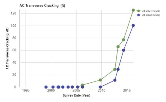
Figure 11. Total transverse cracking (length) observed over time.
