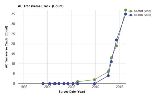
Figure 10. Total transverse cracking (count) observed over time.
