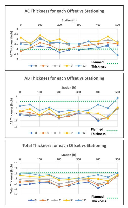
Figure 15. Summary of AC (top), AB (middle), and Total Pavement Thickness (bottom) for test section 35\_0801, with the green line representing the planned thickness for each layer.
