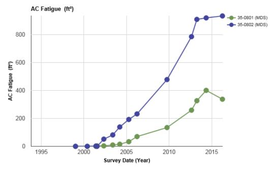
Figure 6. Total area of alligator cracking over time.
