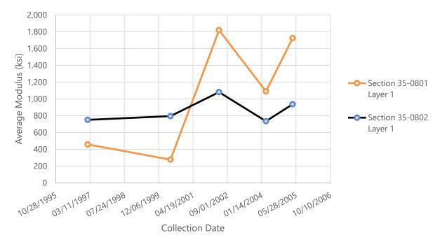
Figure 2. Average modulus of AC layers for test sections over time.
