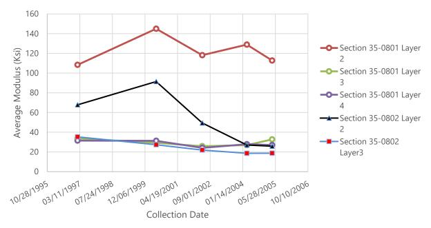
Figure 3. Average modulus of base and subgrade layers for test sections over time.
