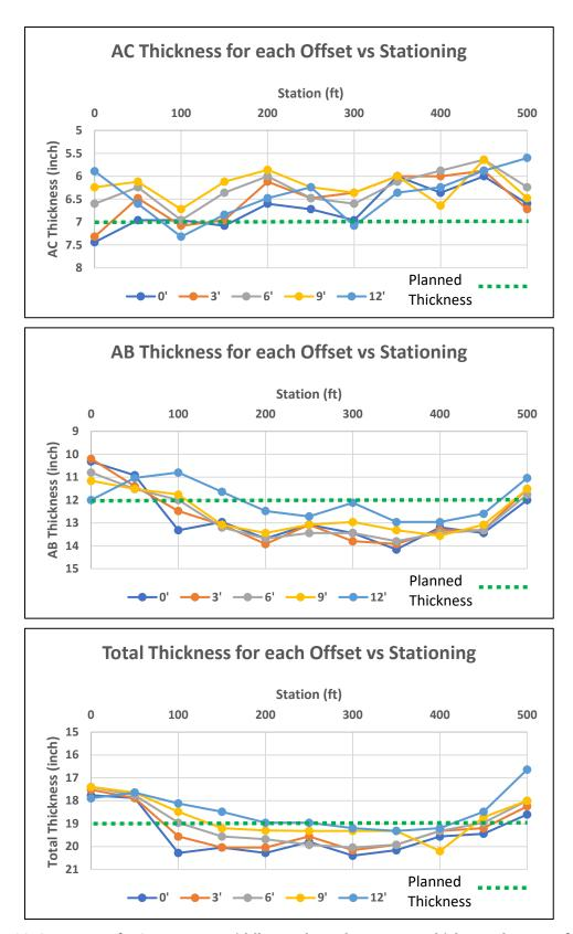
Figure 16. Summary of AC (top), AB (middle), and Total Pavement Thickness (bottom) for test section 35\_0802, with the green line representing the planned thickness for each layer.
