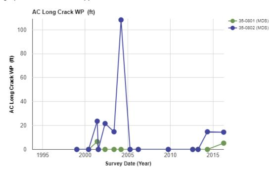
Figure 8. Total longitudinal cracking on the wheelpath over time.
