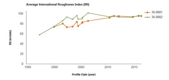
Figure 12. Average pavement roughness over time.
