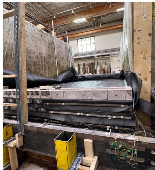
Figure 2.9 Geotextile installation between facing blocks
