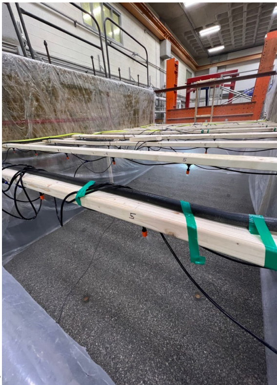
Figure 2.15 Wooden frame to support backfill sprinkler system
