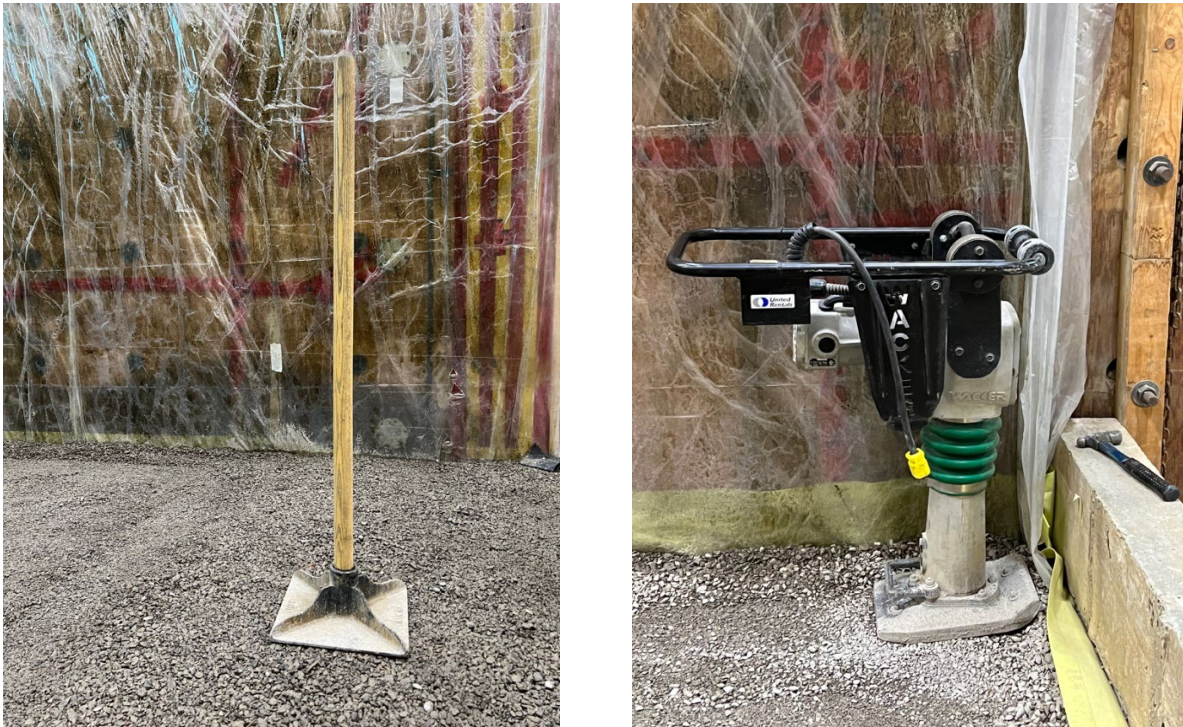
Figure 2.10 Compaction equipment: (a) hand tamping compactor and (b) lightweight jumping jack tamper compactor
