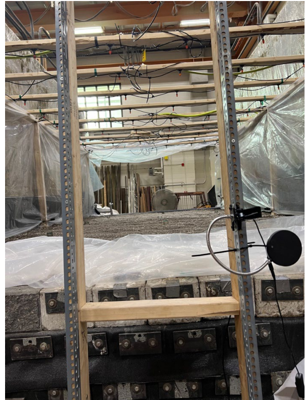
Figure 2.15 Wooden frame to support backfill sprinkler system
