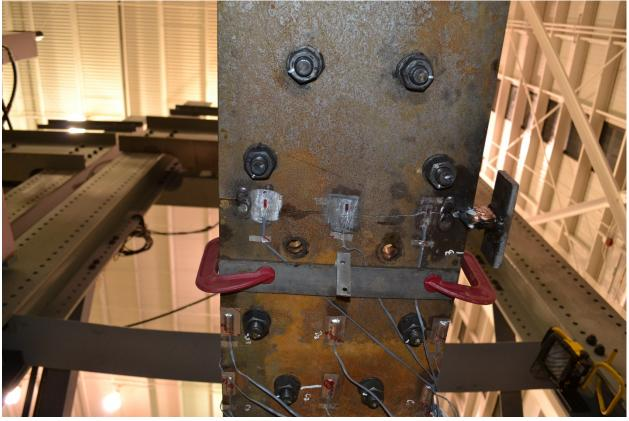
Figure 3: View looking up at fractured cover plate of specimen 46-4
