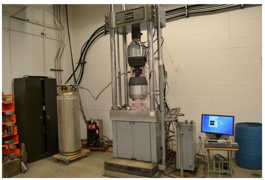
Figure 1: Test setup for evaluating of brittle weld fracture method
