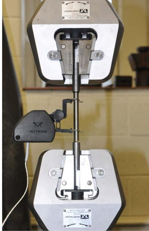
**Figure 2-8. Tensile Test Specimen with Extensometer**
