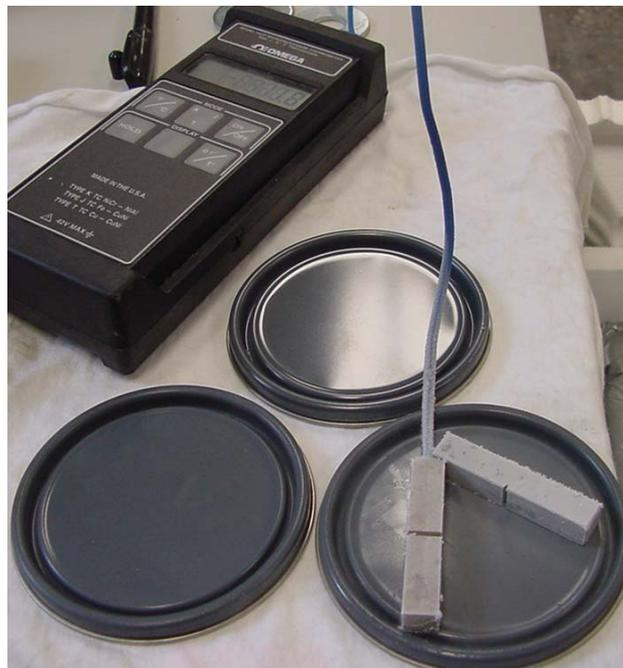
**Figure 2-10. CVN Specimen Reaching Desired Test Temperature**
