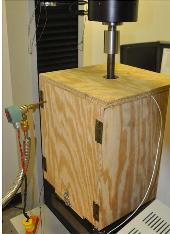
**Figure 2-19. Environmental Chamber on Crack Arrest Apparatus**
