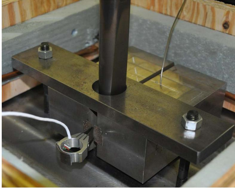
**Figure 2-16. Crack Arrest Specimen Prior to Testing**
