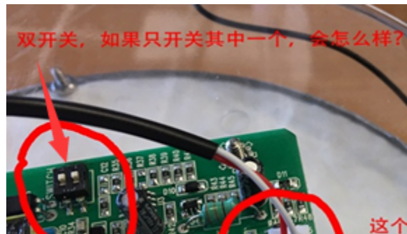
Figure 3 Problem of the double switch on the electronic board of the LED drivers, which is not as reliable as single switch
