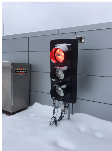
Figure 5 In real-time snowy winter 2019, the closed-course performance and reliability tests of the fully working prototypes mounted on the roof of M2SEC building. The roof tests have been continuously conducted with necessary real-time adjustments.
