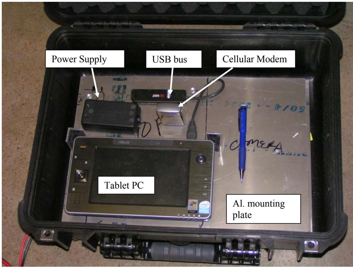
**Figure 1.** Photograph of the prototype FDAS showing the tablet PC, USB bus, power supply and cellular modem.
