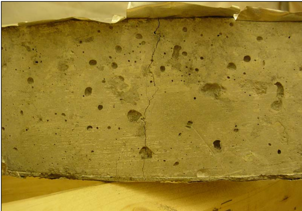
Figure 3.40 - Crack observed in MoDOT Ring A on day 103.
