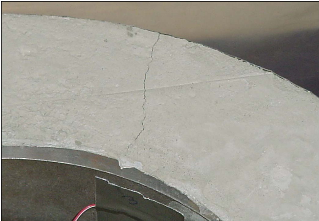
Figure 3.8 - Crack observed in ring P3 on day 6
