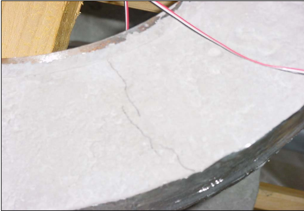
Figure 3.7 - Crack observed in ring P2 on day 27
