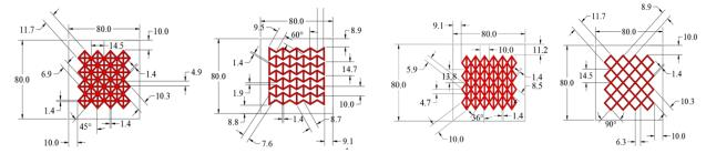
• ISU based on test data, the reinforced pattern (first on left) was selected to move forward and replace the nontextured SEC. This selection was based on the higher linearity of the CGI vs crack length results (figure below) and symmetry of the pattern that results in an easier field deployment.
