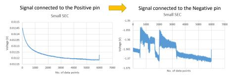
• KU identified issues 2 (linear drift) shown below, which was due to the power of the Xnode. It can be solved through signal processing.
