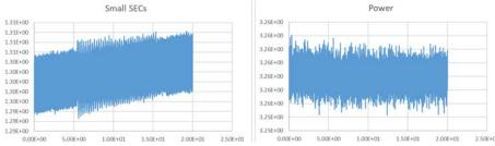
• KU identified issues 3 (long-period signal fluctuation) as shown below. The long-period fluctuation occurred when multiple SEC sensors with their UA boards were connected and powered by one Xnode. The solution is still being investigated.
