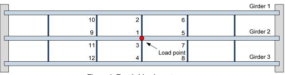
Figure 1: Test bridge layout
