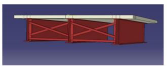
Fig. 4. Exposed view of lateral bracing at mid-span
