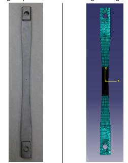
Fig. 10. Fatigue specimen with undersized crack-stop hole
