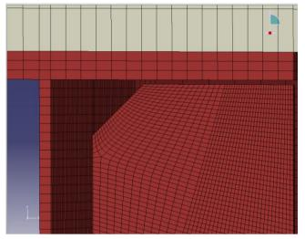
Fig. 5. View of clipped connection stiffener at the top flange
