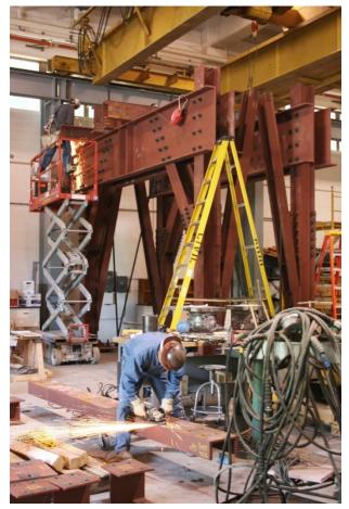
Fig. 1. Test frame under construction
