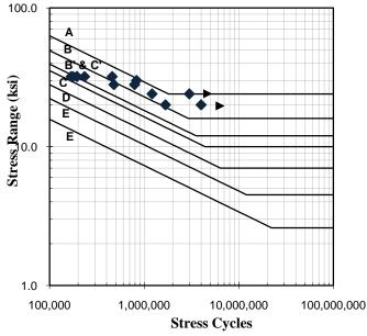
Fig. 9. SN Diagram showing performance of control specimens
