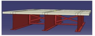
Fig. 3. View of overall model of three girder bridge assemblage
