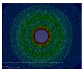
Fig. 12. Von Mises residual stress fields for 3% expansion of crack-stop hole
