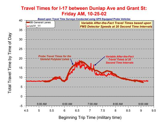
Fig. 2.7: Example of After-the-Fact Travel Time Compared to Observed Probe Travel Time
