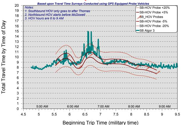
Fig. 2.14: Comparison of the Results of the Predictive Travel Time Algorithm with Comparable Observed Travel Times for Southbound HOV Lanes
