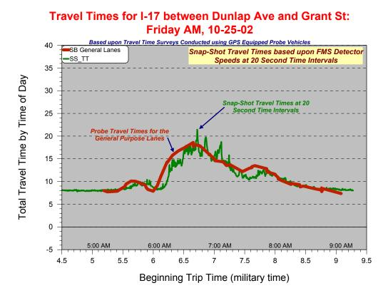
Fig. 2.6: Example of Snap Shot Travel Compared to Observed Probe Travel Time
