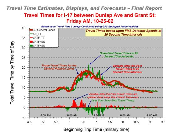
Fig. 2.8: Example of Comparison of Snap Shot Travel Time to After the Fact Travel Time
