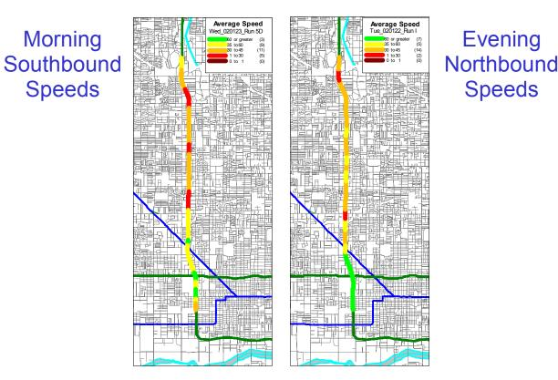
Fig. 2.2: Avg. Speed Between Detectors based on GPS Data
