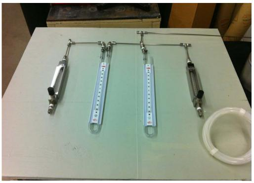
Figure 12: Swiss Permeability instrument
