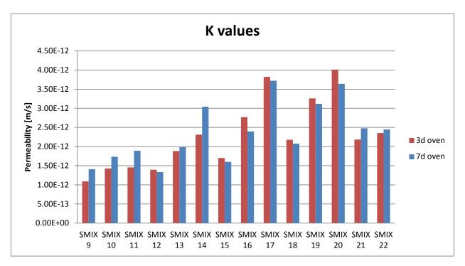
Figure 6: Permeability – Sulfate mixtures
