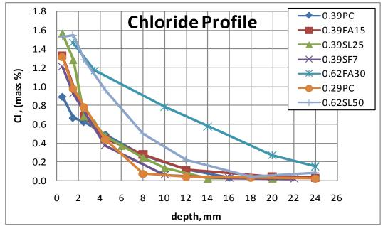
Figure 9. Chloride Profile (ASTM C1556) for 56d normal curing followed by 21 week in cyclic exposure
