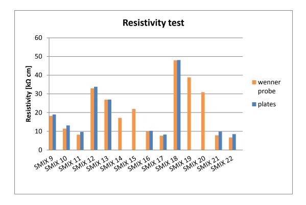
Table 5: Resistivity results – Freeze and Thaw mixtures ( $k\Omega$  cm)
