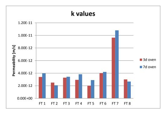
Figure 8: Permeability – Freeze and Thaw mixtures
