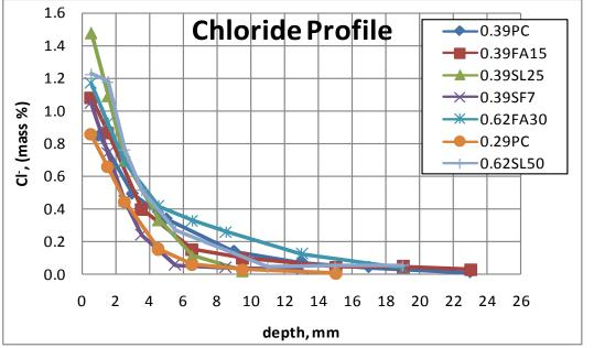
Figure 7. Chloride profile for 56d normal curing followed by 35d in solution
