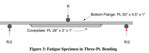
(Figure 3) consist of two-plate assemblies representative of a bottom flange and a welded cover plate loaded in three-point bending. A total of fifteen specimens are being tested to evaluate the increase in fatigue life obtained by using the two retrofit measures separately and in combination.
