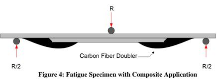
or "fuses". Figure 4 depicts the fatigue specimens outfitted with the composite doublers.
