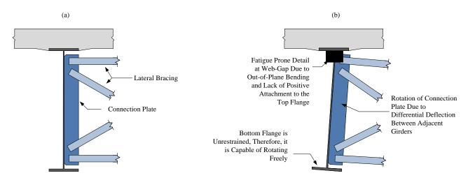
Figure 1: (a) Girder Cross-Section before Differential Displacement (b) Girder Cross-Section after Differential Displacement
