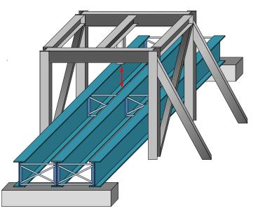
Figure 5: Test Set-up for Loading Girder System
