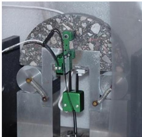
**Figure 6.7: The SCB test**
