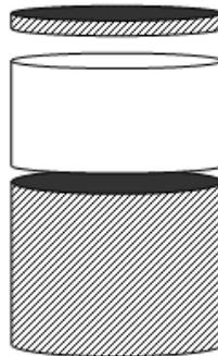
**Figure 3.4: Sample preparation for field cores**
