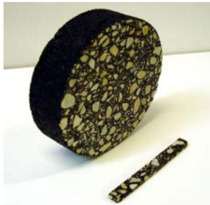
**Figure 9.2: IDT and BBR test specimens**
