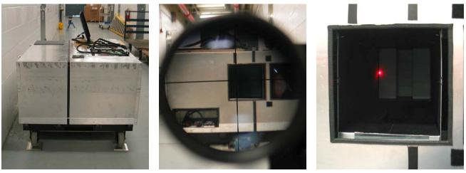
a. Profiler on leveling shims 30 ft. in front of the laser
