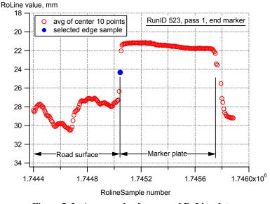
Figure 5. 2. An example of processed RoLine data in the vicinity of an end-marker plate
