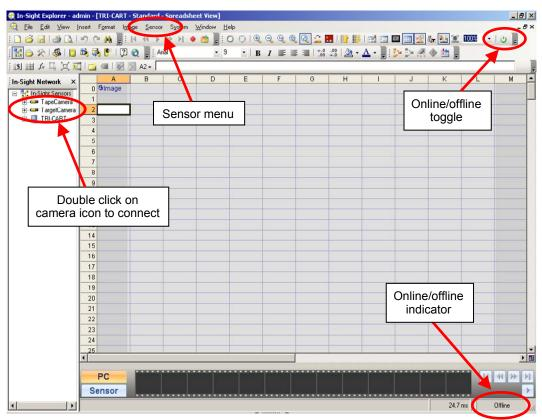
Figure B.8. *In-Sight Explorer* screen on start up (Spreadsheet view)
