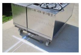
Figure 4.9. The profiler in position to start the measurement of a segment
