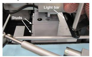
c. Take care that the battery is clear of the light bar and the studs; lower the battery jack.
