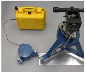
Position the assembly & power up Position using the alignment plate. Rotate the mounting dish to aim. Lock the mounting plate. Connect cables & turn on switches.
