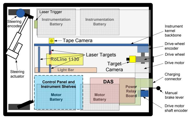
Figure 1.3. A schematic diagram of the major elements of the benchmark profiler in plan view
