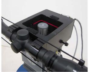
b. Rear quarter view showing the laser beam sweeping across the window into the circuit camber
