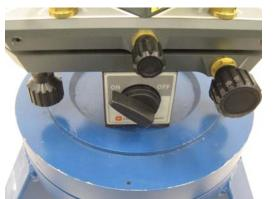
a. The L-740 properly mounted: the front corners of the magnetic base are firmly against the edge of the dished surface and the magnet switch is on.
