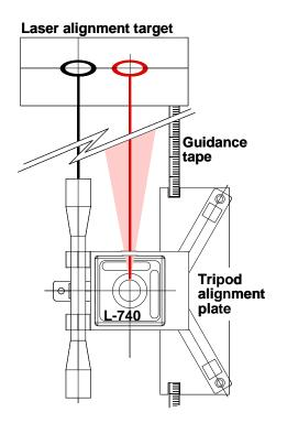
Figure 3.7. A schematic diagram of the lateral and yaw alignment of the spinning laser
