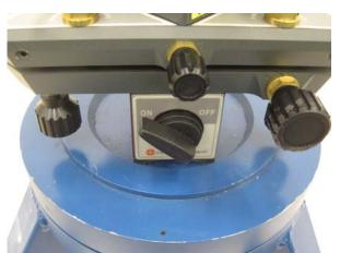
1. Position of the laser on the tripod The corners of the magnetic base firmly against the edge of the dished surface and the magnet switch on.
