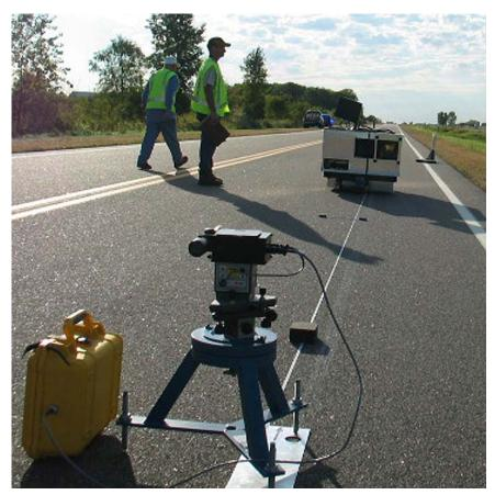
Figure 1.1. The benchmark profiler tracking the guidance tape autonomously with the spinning laser in the foreground
