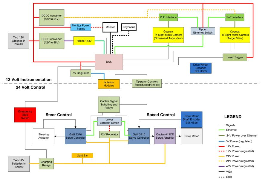
Figure F.2. Block diagram of the electrical systems
