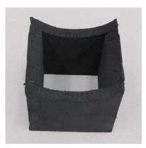
Figure A.15. Sun shade for laser bubble-levels
