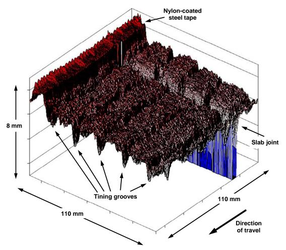
Figure 1.7. Surface plot of RoLine measurements of a new, longitudinally-tined road surface 314 lines x 150 points/line = 47,100 points
