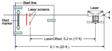
Figure 2.7. The initial laser offset for the standard test setup is 5.2 m.
