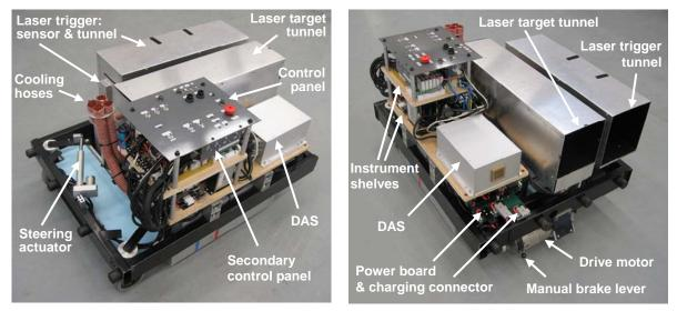
b. With the cover removed, from the left front c. With the cover removed, from the left rear Figure 2.1. Three views of the benchmark profiler showing the location of its controls and major components
