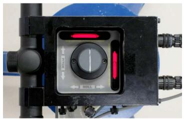
Figure 3.9. Top view of the spinning laser with bubble levels illuminated. The roll bubble is well centered; the pitch bubble is off center.
