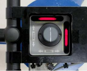
**4.** Level the laser in roll. Use the roll adjustment and the roll bubble level to level the laser in roll. Repeat after step 5.
