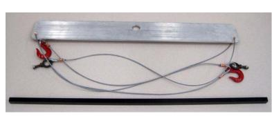
Figure A.20. Lifting hardware: spreader, cables and crossbar
