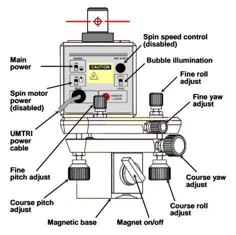
Figure 3.3. A sketch of the modified HAMAR L-740 spinning laser (rear view)
