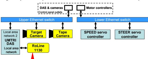
Figure B.1 provides a simple schematic of the three Ethernet networks of the benchmark profiler.
