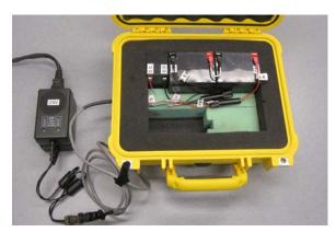
a. The battery pack with chargers and three batteries b. The chargers removed for charging the batteries Figure 3.11. The battery pack for the spinning laser system
