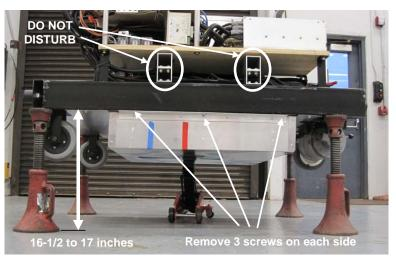
Figure D.3. The benchmark profiler supported on four post jacks with the battery jack <u>lightly</u> supporting the center floor panel
