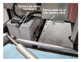
Figure D.4. View of the batteries on the right side (8-in., 12-volt system) looking from the front
