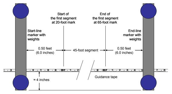
Figure 4.7. Placement of the start-line and end-line marker strips for the first segment (not to scale)
