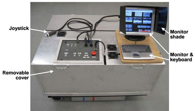
a. With cover, joystick, monitor & keyboard, and monitor sun shade
