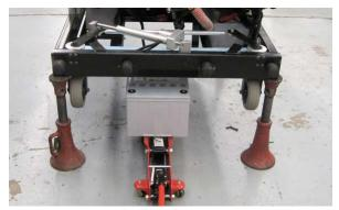
d. Rotate the jack 90 degrees and remove it and the battery toward the front of the profiler.
