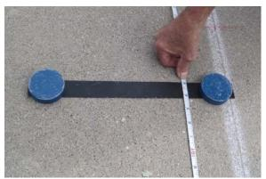
Figure 4.12. Aligning the 19.50-ft. mark of the guidance tape with the edge of the start-line marker.
