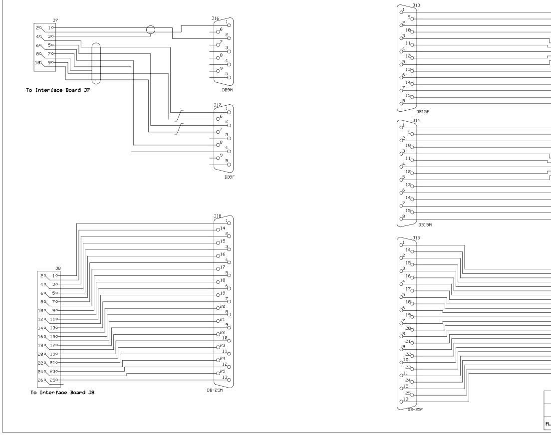
Figure F.14. Cart – DAS internal wiring; 1 of 2
