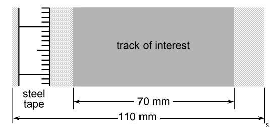
Figure 1.6. Layout within the RoLine footprint
