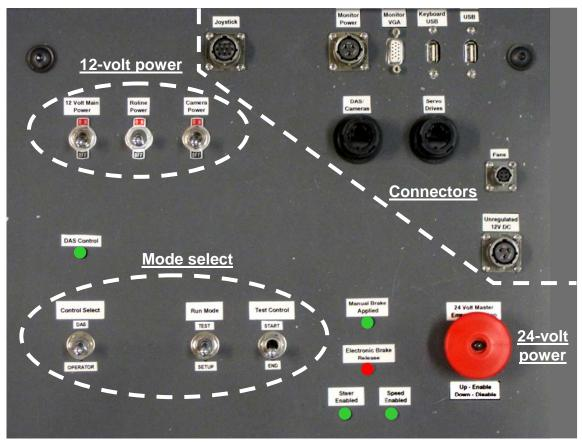
Figure 2.2. The benchmark profiler's control panel (with group indications added)
