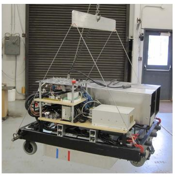
Figure D.2. The benchmark profiler suspended from an overhead crane using the special lifting hardware
