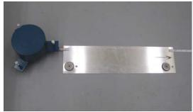
Figure 3.5. Tripod alignment plate positioned over the guidance tape
