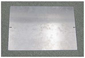
Figure A.14. Marker-strip transfer plate
