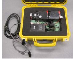
b. Open showing batteries and chargers a. Battery pack closed Figure A.9. Laser battery pack
