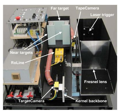
Figure 1.4. Features of the instrument kernel and the laser trigger
