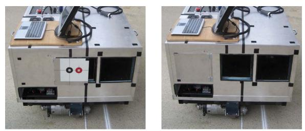
a. Target displayed b. Target stowed Figure 4.8. The laser alignment target on the rear of the benchmark profiler
