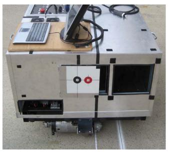
Figure 3.8. The laser alignment target, in the display position, on the rear of the benchmark profiler
