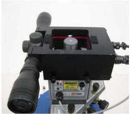
Position of the shroud on the laser. Laser controls to the rear. Sighting scope to the left; four thumbs screws firmly tightened.
