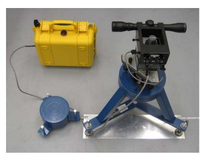
Figure 3.1. The spinning laser assembly, with battery pack, positioned over the guidance tape with the tripod alignment plate
