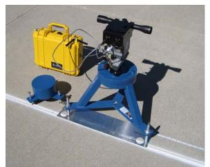
Figure 4.10. The spinning laser in position at the start of the guidance tape
