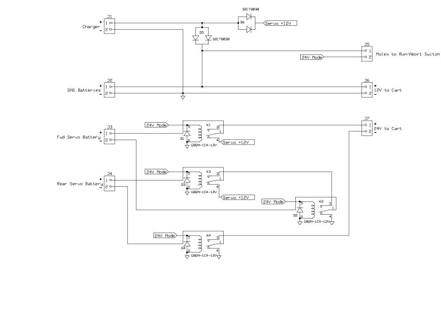
Figure F.9. Cart – Power relay board
