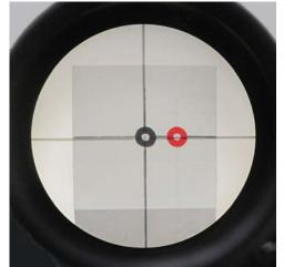
5. Align the laser in pitch and yaw. Use the pitch and roll adjustments and the sighting scope to align the laser in pitch and yaw. <u>Repeat step 4.</u>
