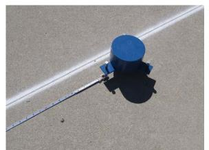
b. The start of the guidance tape anchored with the weighted tripod.
