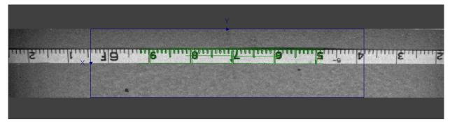
Figure 1.9. An example image from the TapeCamera with trained-pattern match
