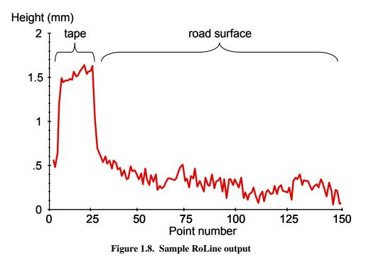
The 95 points within the track of interest are reduced to a single range value using a bridging filter. The filter establishes height within the line of interest by seeking the elevation that would produce an average "penetration" upward of 0.7 mm. Thus, the filter is sensitive to positive texture, but it ignores narrow downward spikes within each line of output from the RoLine.
