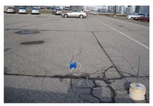
c. The far end of the stretched rope anchor with the second anchor plate and vehicle
