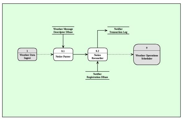
Figure B-21 Pooled Fund MDSS STWx Level 2 Data Flow Diagram for the Data Notifier Process
