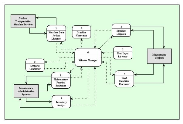
Figure B-2 Pooled Fund MDSS Level 1 Data Flow Diagram
