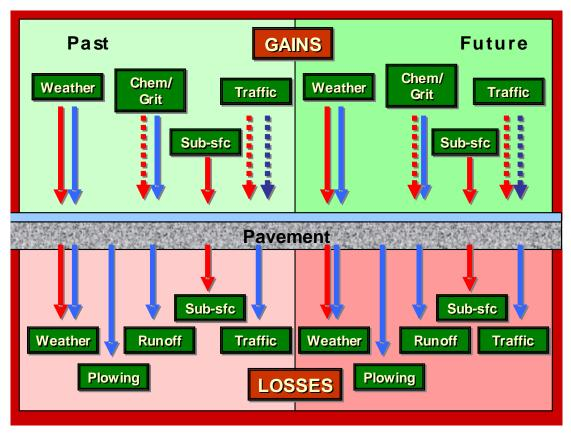
Figure 7-3 Schematic Depiction of Factors Associated with Pavement Condition and Its Change as Found within the Pooled Fund Study Approach
