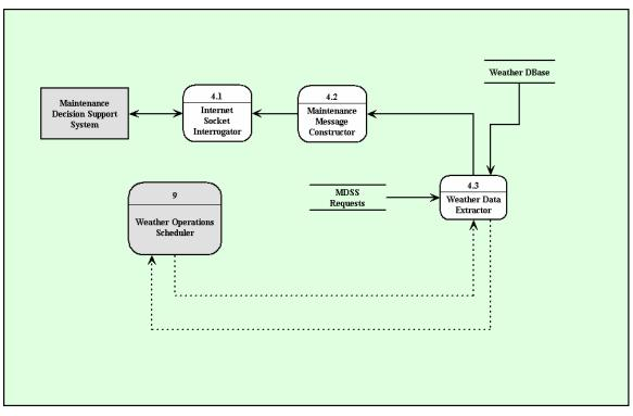
Figure B-17 Pooled Fund MDSS STWx Level 2 Data Flow Diagram for the Surface Transportation Weather Packager Process
