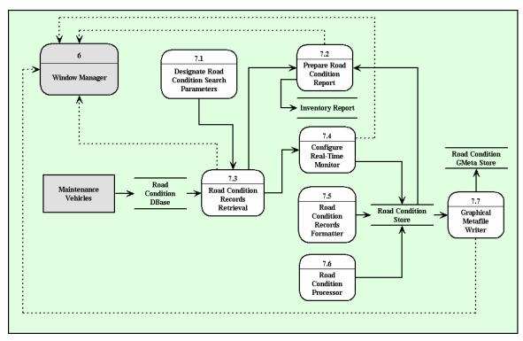
Figure B-9 Pooled Fund MDSS Level 2 Data Flow Diagram for the Road Condition Processor
