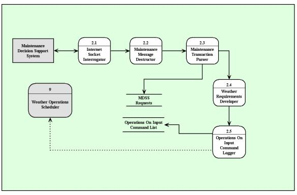
Figure B-15 Pooled Fund MDSS STWx Level 2 Data Flow Diagram for the Maintenance Transaction Listener
