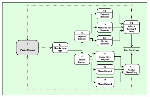
Figure B-4 Pooled Fund MDSS Level 2 Data Flow Diagram for the User Input Listener Process
