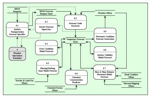
Figure B-19 Pooled Fund MDSS STWx Level 2 Data Flow Diagram for the Surface Transportation Forecast Generator Process
