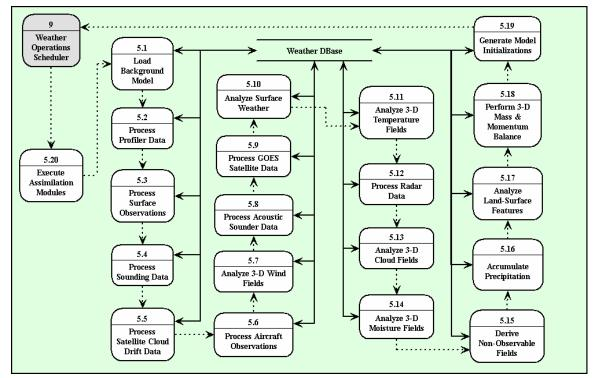
Figure B-18 Pooled Fund MDSS STWx Level 2 Data Flow Diagram for the Weather Data Assimilation Process
