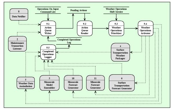
Figure B-22 Pooled Fund MDSS Level 2 Data Flow Diagram for the Weather Operations Scheduler Process
