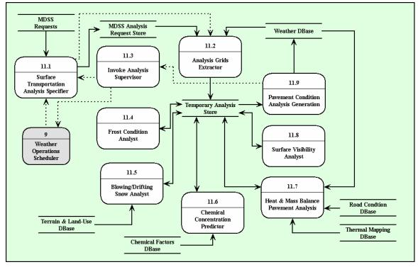
Figure B-24 Pooled Fund MDSS STWx Level 2 Data Flow Diagram for the Surface Transportation Analysis Generator Process
