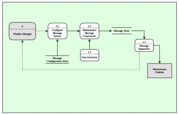
Figure B-6 Pooled Fund MDSS Level 2 Data Flow Diagram for the Message Dispatch
