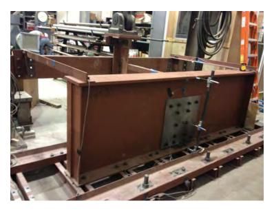
Figure B.68: View on the exterior face of the girder's web with a steel back plate
