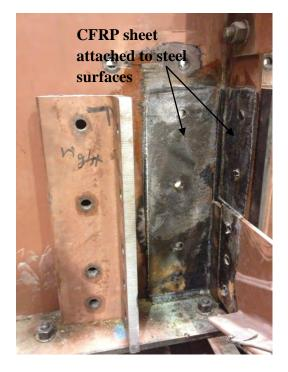
Figure B.71: Trial 2: view of the interior face of the girder's web
