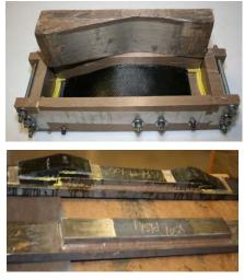
Figure B.21: Three point bending specimens (a) Test setup; (b) CFRP overlay in fabrication mold; (C) Unreinforced and reinforced specimens side by side.
