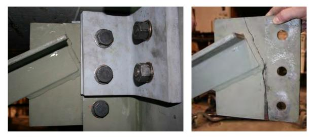
Figure A.33: North cross frame failure during Trial 4N
