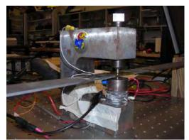
Figure C.4: Photograph showing PICK tool being used to treat a crack stop hole in a steel fatigue specimen
