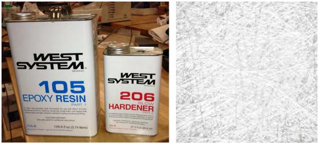
Figure B.40: Materials used in the FRP block (a) West System™ two-part epoxy; (b) Mat fiberglass
