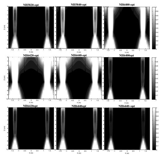
FIGURE 5. Damage factor contours for all the study mixtures after five years.
