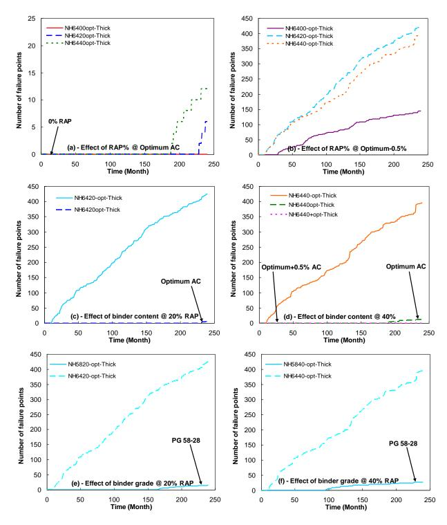
2 FIGURE 7. Evaluation of the effects on thick pavement fatigue life predictions: (a) RAP
