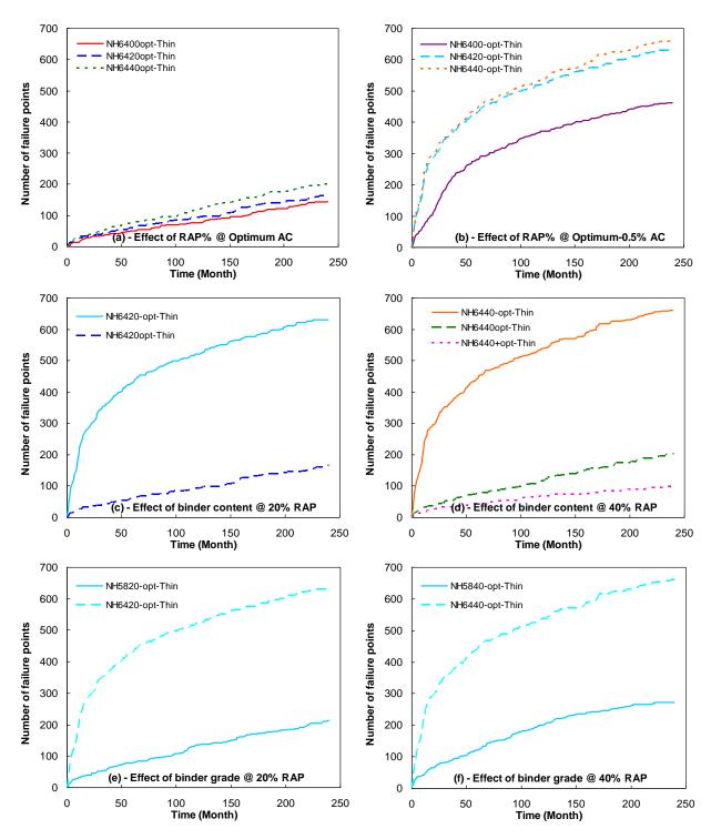
2 FIGURE 6. Evaluation of the effects on thin pavement fatigue life predictions: (a) RAP
