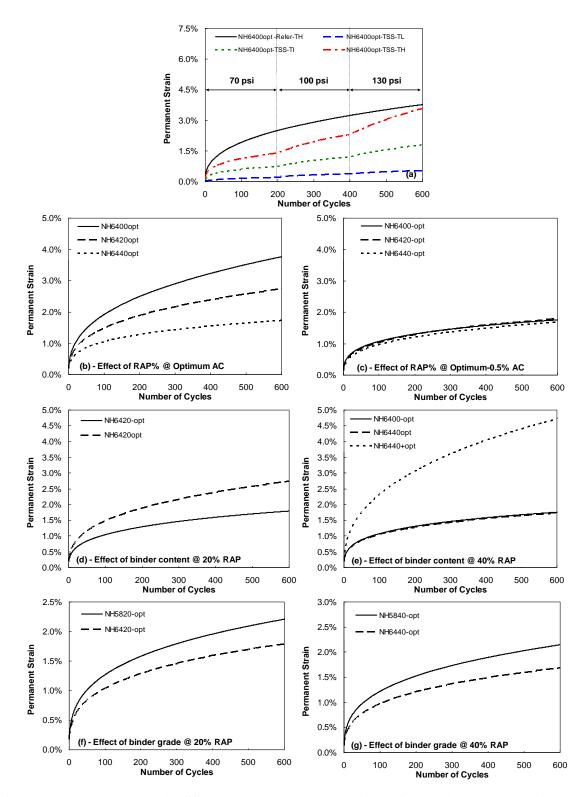
2 FIGURE 4. (a) Example of TSS test results, and evaluation of the effect on the mixture
