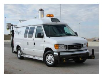
Figure 2.16. Pathway multi-function data collection equipment.
