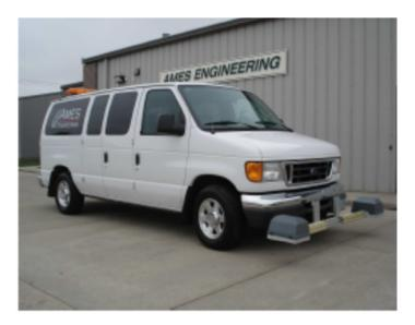
Figure 2.5. Portable profiler mounted on the front of a van.
