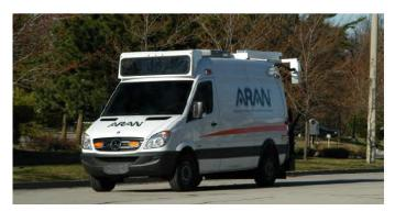
Figure 2.13. Fugro-Roadware multi-function data collection equipment.
