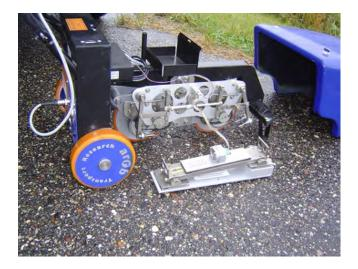
Figure 2.6. ARRB walking profiler.
