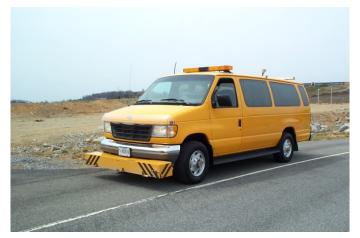
Figure 2.2. High-speed profiler.
