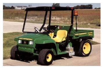
Figure 2.3. Lightweight profiler.
