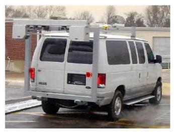
Figure 2.12. Dynatest multi-function data collection equipment.
