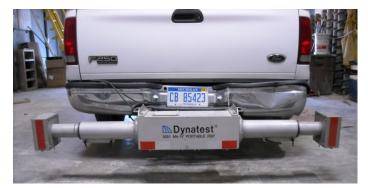
Figure 2.4. Portable profiler mounted on the back of a vehicle.
