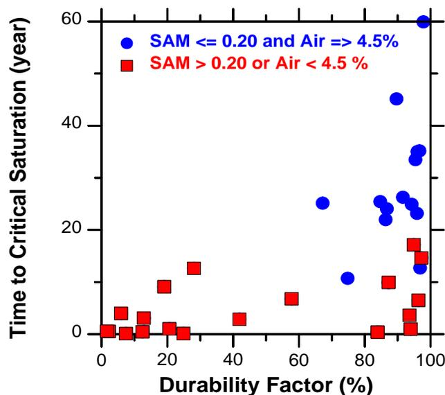
Figure 1 – Time to critical saturation as determined by the bucket test is shown versus the ASTM C 666 durability factor. Good agreement is shown between the two methods.
