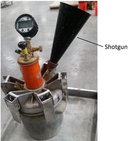
**Figure 2.4.2 – A funnel and threaded tube that allows water to be continuously added to the bottom chamber while filling.**
