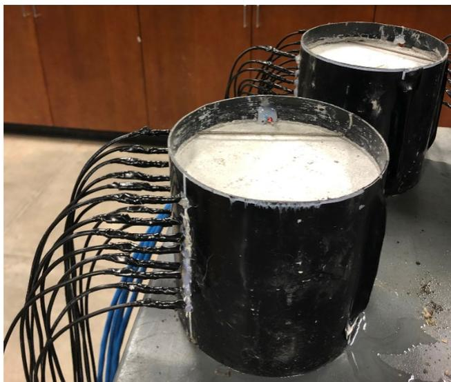
**Figure 3.4.3. Mortar sample molds.**
