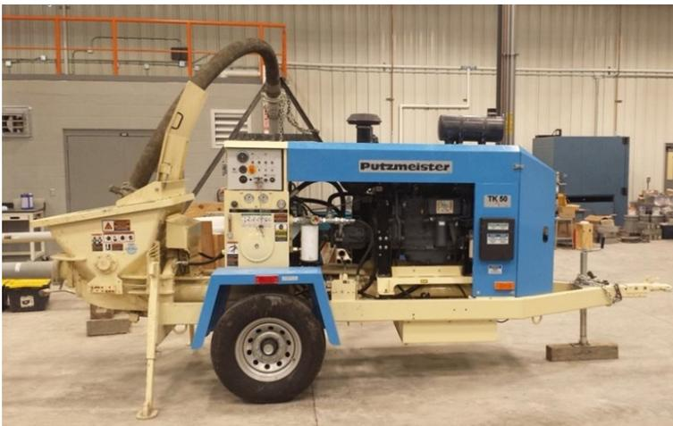
Figure 2.5.1. The Putzmeister TK 50 Concrete Pump used for all laboratory testing.
