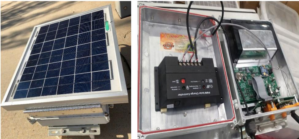
**Figure 3.4.5. Instrument box with solar panel**
