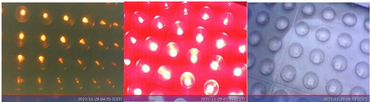
Figure 6 Michigan field test data collected in November 2021 after the field installation on November 4 th , showing the normal performance of the red, yellow, and green signal lights under mild and cold weather conditions. Note that before Nov 17, 2021, the green signal light had higher lens surface temperature due to its longer power-on timing than red signal light. This timing sequence was changed after Nov 17 per our request to keep the green and red signal with well-balanced power-on timing, resulting in close temperature measured on the lens surface for both green and red light.
