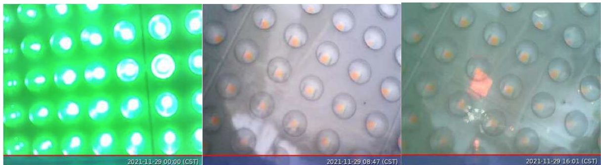
Figure 4 Wisconsin field test data collected in November 2021 after the field installation on November 3 rd , showing the normal performance of the red, yellow, and green signal lights under mild and cold weather conditions, especially for the green signal light which had the longest power-on time. Note that due to traffic demand in the early morning before sunrise, the green signal light was remained always powered on at that intersection while red and yellow signals were rarely powered on, resulting in a large temperature gap between the green signal lens and the ambient air, with minimal heat buildup on the red and yellow signal lenses during the traffic control period (midnight - sunrise).
