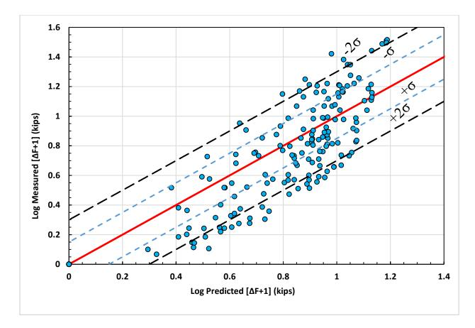
Figure 3-12: Logarithm of measured induced tensile force plus one for data obtained from fixed head conditions test vs logarithm of predicted induced tensile force plus one using Equation 3-4.
