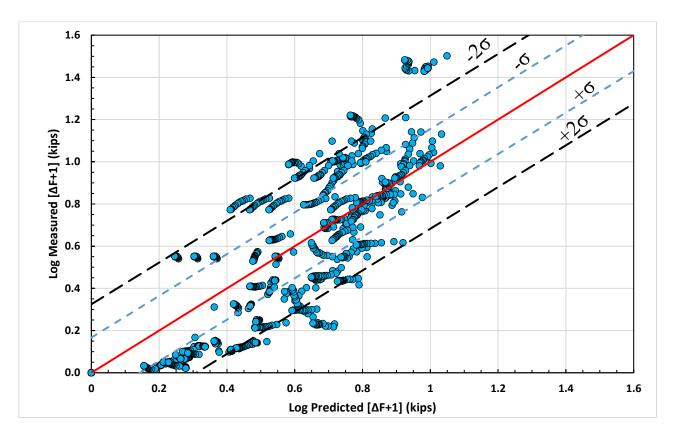
3-4 with the data obtained from maximum tensile force measured for cyclically loaded piles towards the wall.
