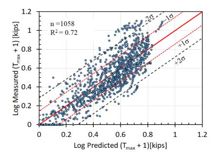
Figure 2-6. Predicted versus measured maximum welded wire reinforcement tensile force (Luna, 2016)
