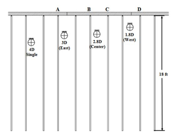
Figure 2-11. Location of ribbed strip reinforcements and the piles that were tested as a group (Farnsworth, 2020).
