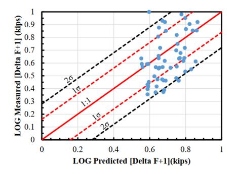
Figure 2-8. Statistical comparison of previously suggested equation for prediction of tensile force experienced by the soil reinforcements and the measured tensile force by ribbed strip reinforcements. (Wilson, 2020).
