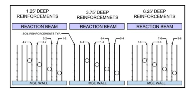
Figure 2-7. Map of the soil reinforcements near the 24-inch piles. (Wilson, 2020)
