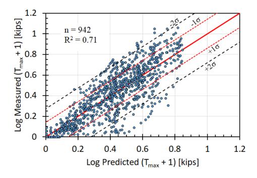
Figure 2-5. Predicted versus measured maximum ribbed strip reinforcement tensile force. (Luna, 2016)
