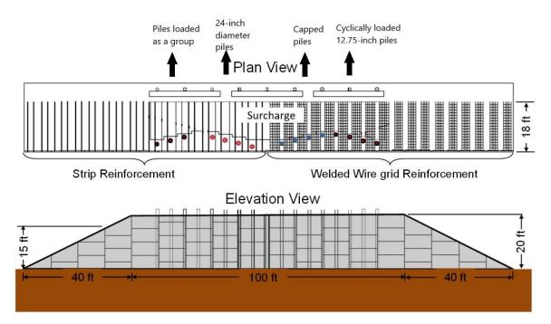
Figure 2-2. Plan view of the MSEW for phase 3
