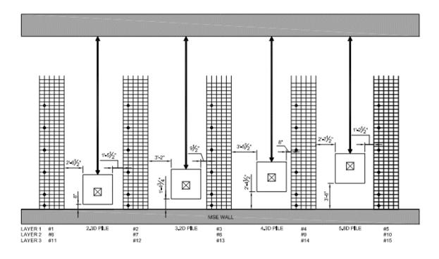
Figure 2-9. Location of the strain gauges in the welded wire reinforcements for fixed head test piles.
