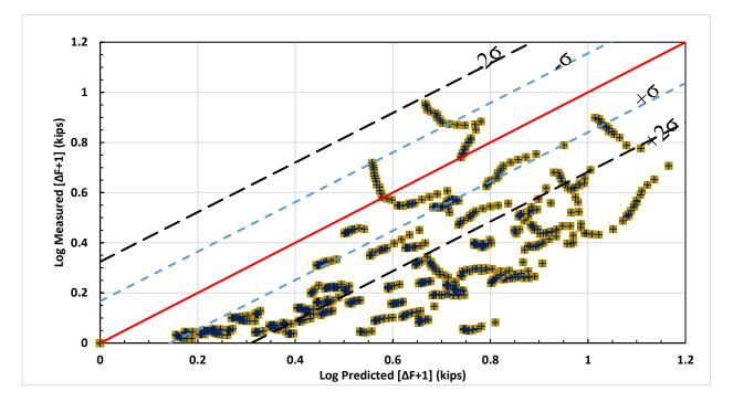
Figure 3-31: Logarithm of measured induced tensile force plus one vs logarithm of predicted induced tensile force plus one using equation 3-4 with cyclic loading away from the wall test data.
