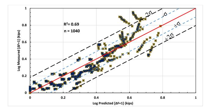
Figure 3-32: Logarithm of measured induced tensile force plus one vs logarithm of predicted induced tensile force plus one for cyclic loading away from the wall.
