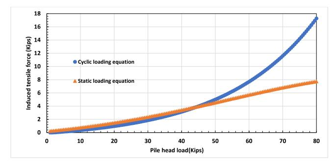
Figure 3-20: Comparison of induced tensile force with static loading equation and cyclic loading equation for a S = 2D
