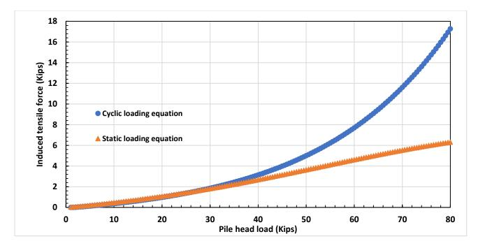
Figure 3-22: Comparison of induced tensile force with static loading equation and cyclic loading equation for a S = 4D
