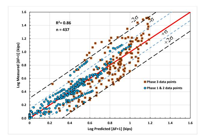
Figure 3-17: Logarithm of measured induced tensile force plus one vs logarithm of predicted induced tensile force plus one for welded wire with 95 percent or more relative compaction.
