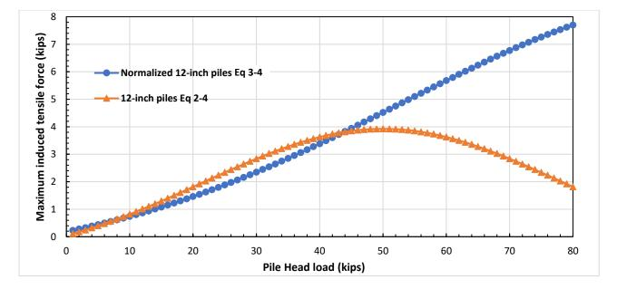
Figure 3-14: Comparison of maximum induced tensile force calculated with equation 3-4 and equation 2-4 for an increasing pile head load.
