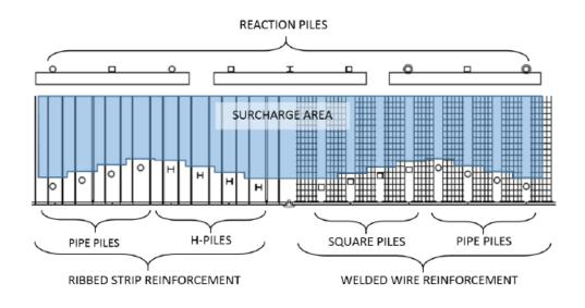
Figure 2-1. Plan view of the MSEW for Phase 1 test loads (Luna, 2016)
