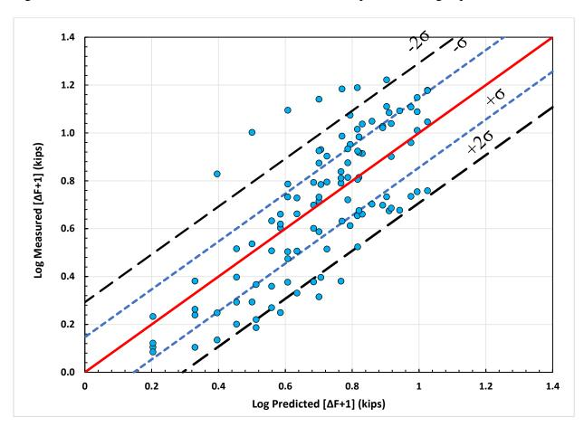
10 shows the logarithm of measured maximum induced tensile force plus one in kips vs the logarithm of the calculated maximum induced tensile force plus one using Equation 3-3.
