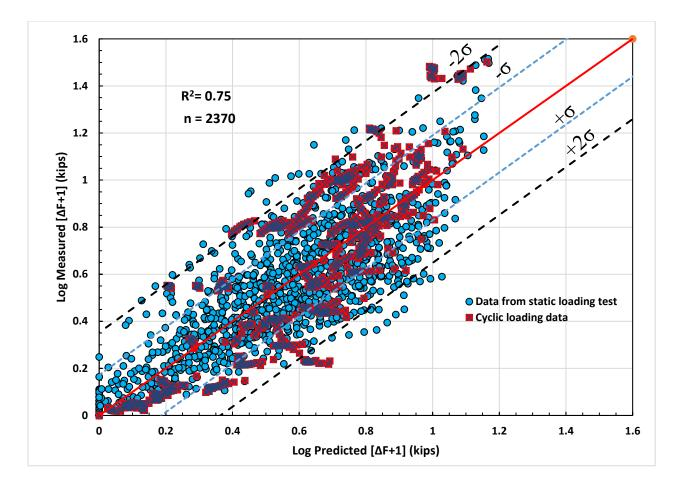
Figure 3-27: Logarithm of measured induced tensile force plus one vs logarithm of predicted induced tensile force plus one using equation 3-9 with all data from tests involving welded wire.
