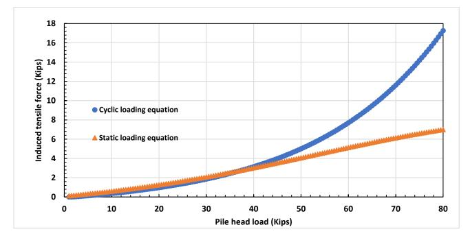
Figure 3-21: Comparison of induced tensile force with static loading equation and cyclic loading equation for a S = 3D
