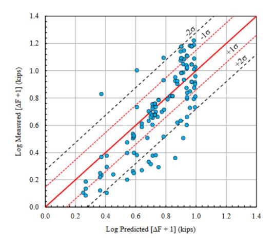
Figure 2-12. Measured versus predicted maximum tensile force in grouped pile soil reinforcements (Farnsworth, 2020).
