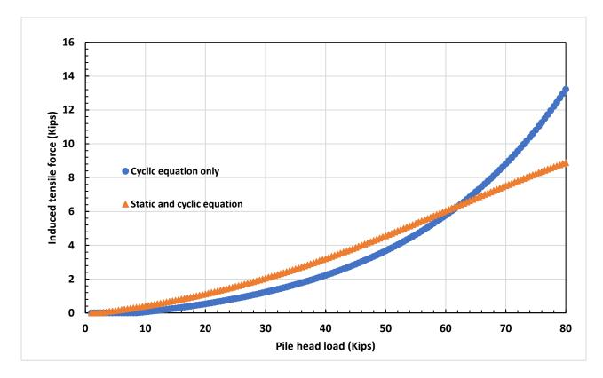
Figure 3-30: Comparison of induced tensile force with static & cyclic loading equation and only cyclic loading data equation for a  $\sigma_v$  at a depth of 6.25 ft
