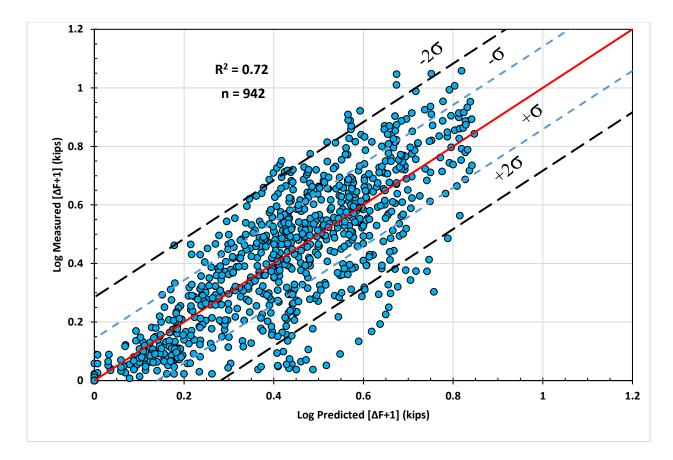
Figure 3-4: Logarithm of measured induced tensile force plus one vs logarithm of predicted induced tensile force plus one comparison for Phase 1 and 2 on ribbed strip reinforcement using dimensionless variables.
