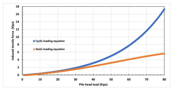
Figure 3-23: Comparison of induced tensile force with static loading equation and cyclic loading equation for a S = 5D
