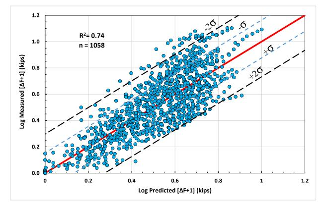
Figure 3-11: Logarithm of measured induced tensile force plus one vs logarithm of predicted induced tensile force plus one comparison for Phase 1 and 2 on welded wire using the dimensionless input variables.
