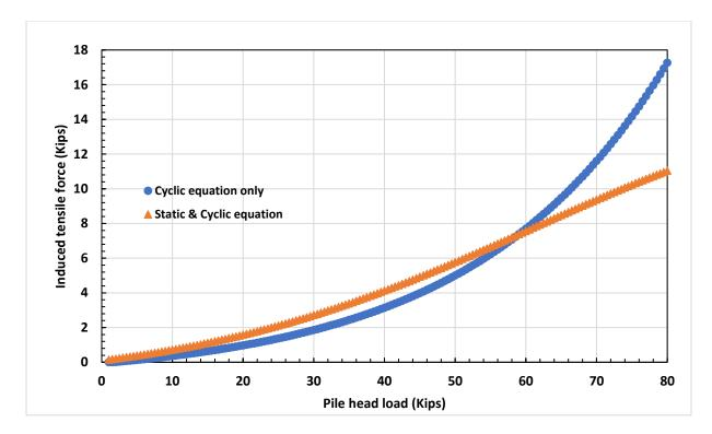
Figure 3-28: Comparison of induced tensile force with static & cyclic loading equation and only cyclic loading data equation for  $\sigma_v$  at a depth of 1.25 ft.
