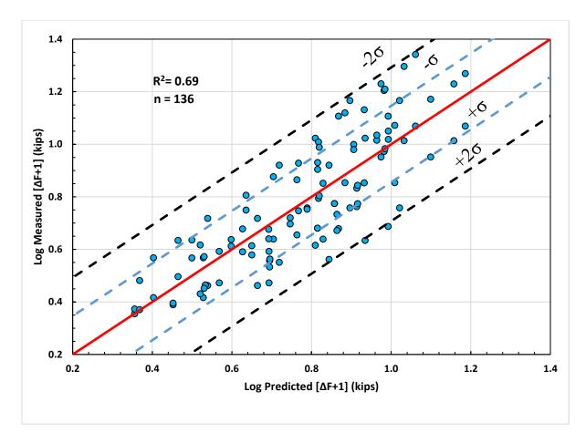
Figure 3-5: Logarithm of measured induced tensile force plus one vs logarithm of predicted induced tensile force plus one in ribbed strip reinforcement comparison for laterally loaded 24" diameter piles behind MSE wall.
