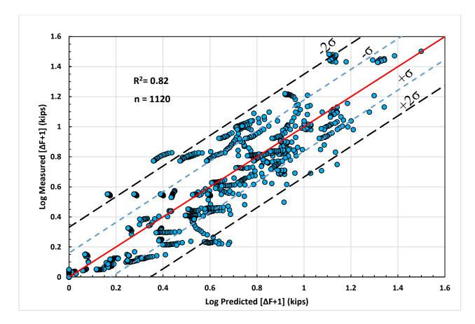
Figure 3-19: Logarithm of measured induced tensile force plus one vs logarithm of predicted induced tensile force plus one using equation 3-8 with cyclically loaded piles towards the wall data.
