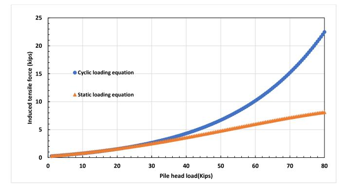
Figure 3-24: Comparison of induced tensile force with static loading equation and cyclic loading equation for a  $\sigma_v$  at a depth of 1.25 ft
