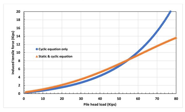
Figure 3-29: Comparison of induced tensile force with static & cyclic loading equation and only cyclic loading data equation for  $\sigma_v$  at a depth of 3.75 ft.
