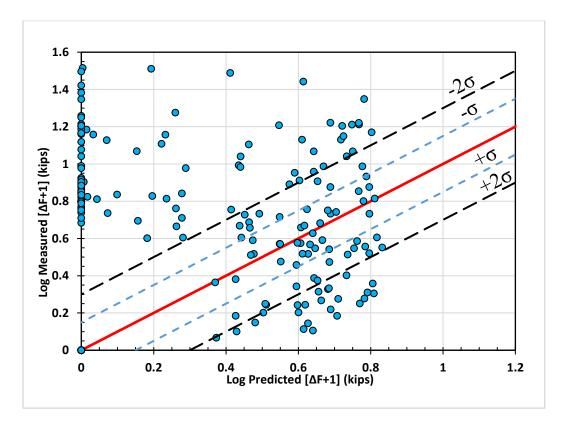
Figure 2-10. Statistical comparison of previously suggested equation for prediction of induced tensile force by soil reinforcements and the measured tensile force by welded wire reinforcements.
