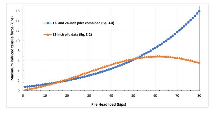
Figure 3-7: Comparison of the maximum induced tensile force calculated with Phase 3 and Phase 1 & 2 prediction equations for a laterally loaded 12.75-inch diameter pile.
