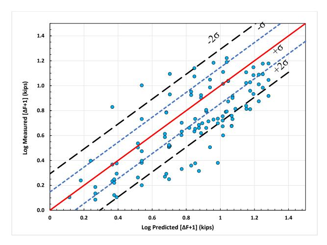
Figure 3-9: Logarithm of measured induced tensile force plus one vs logarithm of predicted induced tensile force plus one comparison using data from group pile test with Equation 3-4.
