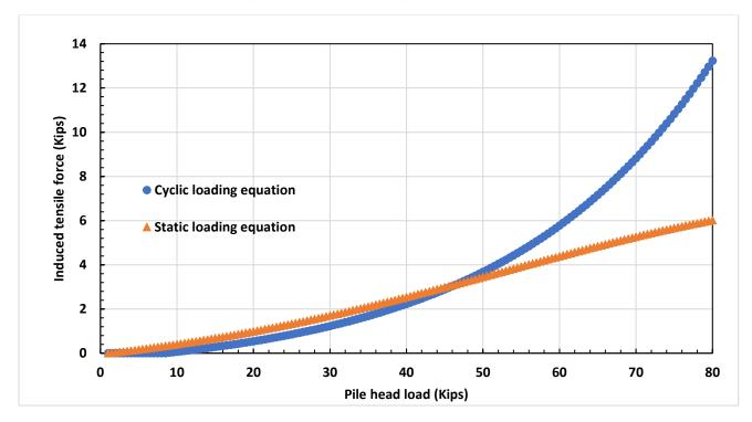
Figure 3-26: Comparison of induced tensile force with static loading equation and cyclic loading equation for a  $\sigma_v$  at a depth of 6.25 ft
