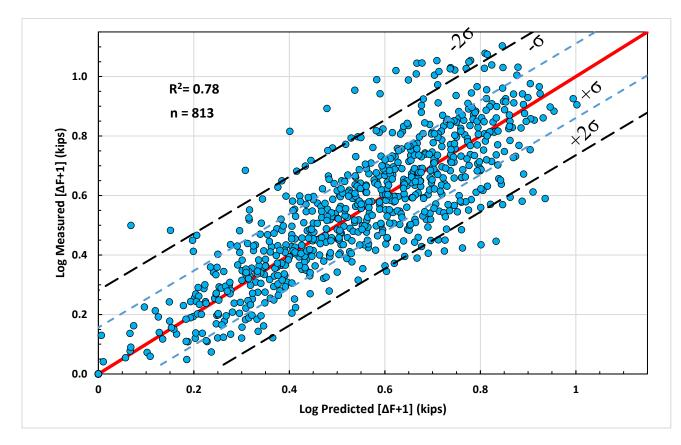
Figure 3-16: Logarithm of measured induced tensile force plus one vs logarithm of predicted induced tensile force plus one for welded wire with less than 95 percent relative compaction.
