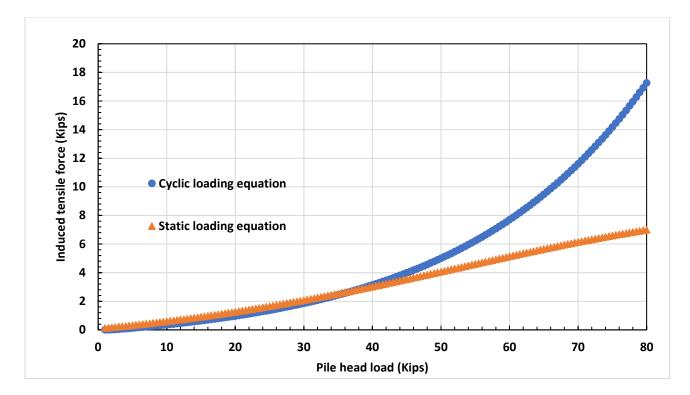
Figure 3-25: Comparison of induced tensile force with static loading equation and cyclic loading equation for a  $\sigma_v$  at a depth of 3.75 ft
