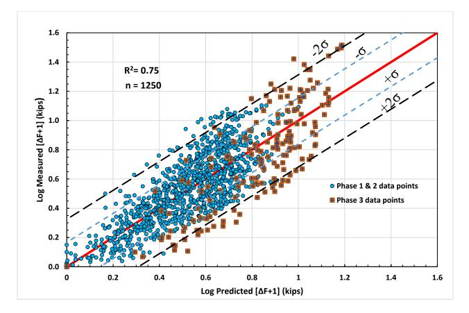
Figure 3-15: Logarithm of measured induced tensile force plus one vs logarithm of predicted induced tensile force plus one using data from all static loading for welded wire data.
