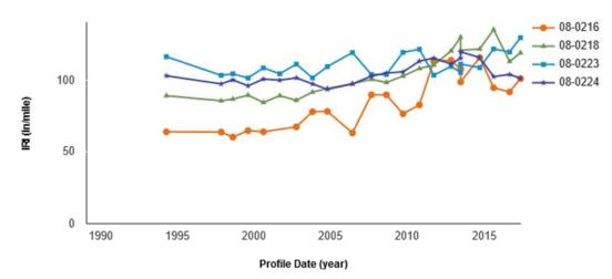
Figure 11. Time history plot of pavement roughness for 080216, 080218, 080223 and 080224.
