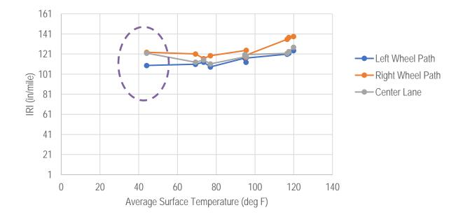
Figure 31. Section 080223 IRI versus temperature, 2019 and 2020 (circled) profile data.
