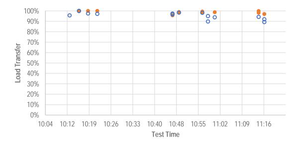
Figure 38. Time history plot of load transfer efficiency at approach (solid orange) and leave (blue) joints for 080224.
