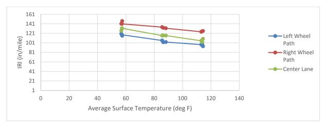
Figure 15. Section 080224 IRI versus temperature, June 23, 2013.
