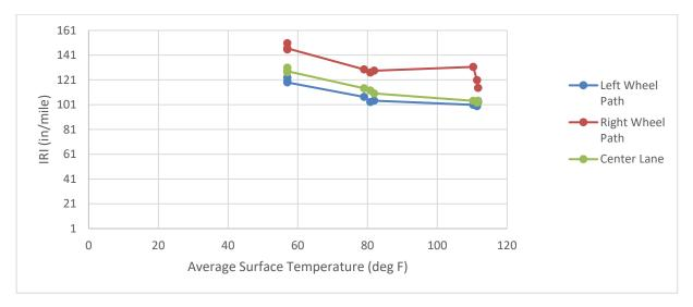
Figure 13. Section 080218 IRI versus temperature, June 23, 2013.
