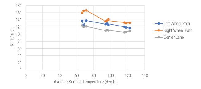
Figure 25. Section 080218 IRI versus temperature, July 13, 2019.
