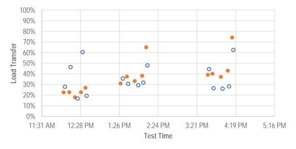
Figure 37. Time history plot of load transfer efficiency at approach (solid orange) and leave (blue) joints for 080223.
