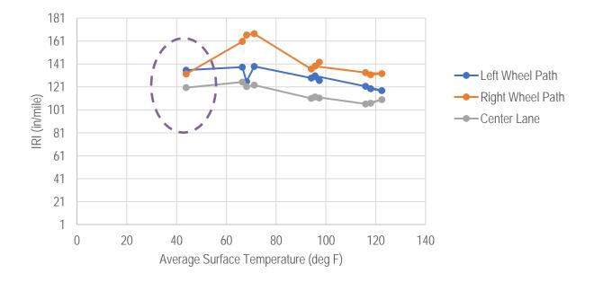
Figure 30. Section 080218 IRI versus temperature, 2019 and 2020 (circled) profile data.
