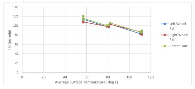
Figure 12. Section 080216 IRI versus temperature, June 23, 2013.
