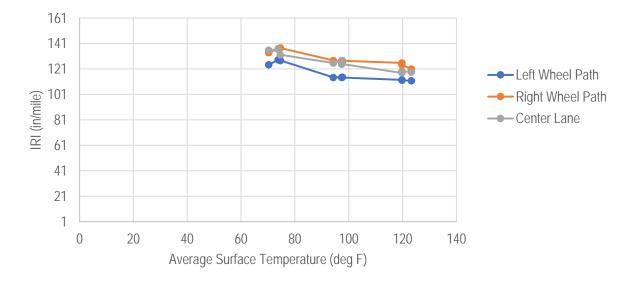
Figure 27. Section 080224 IRI versus temperature, July 13, 2019.
