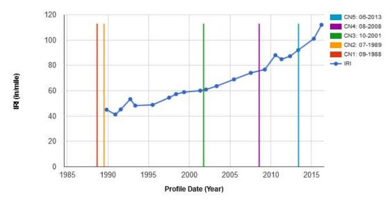
Figure 8. Time history plot of pavement roughness.
