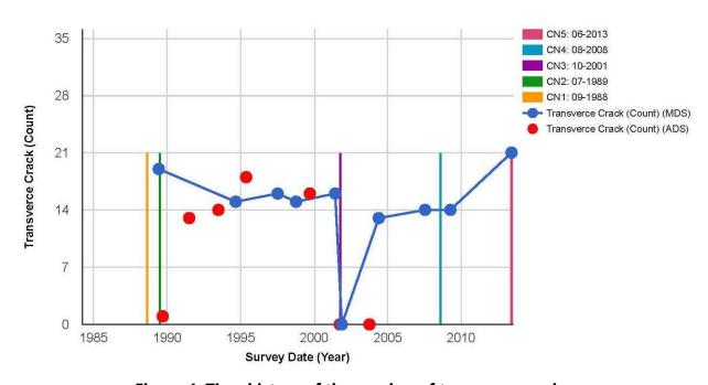
Figure 4. Time history of the number of transverse cracks.
