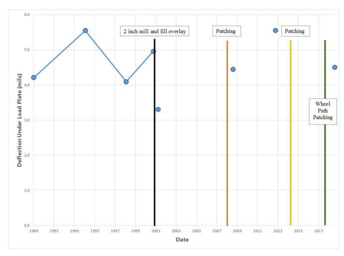
Figure 25. Average FWD wheelpath deflection at the 9,000-lb drop level over time.
