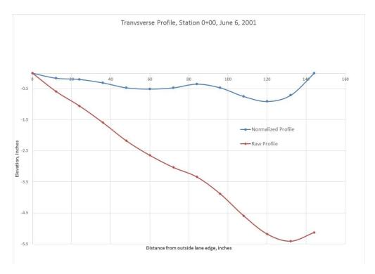
Figure 10. Normalized and raw transverse pavement profile at station 0+00 performed on June 6, 2001 prior to the mill and fill construction event.
