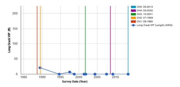
Figure 6. Time history of longitudinal cracking in the wheel path.
