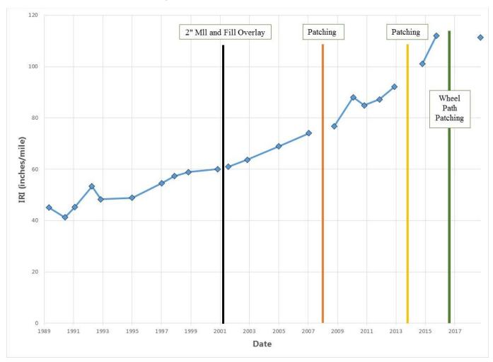
Figure 24. Updated pavement roughness time-history adding the April 2019 LTPP measurement. The wheel path skin patches appear to arrest the further increase in roughness, within the time frame of these measurements.
