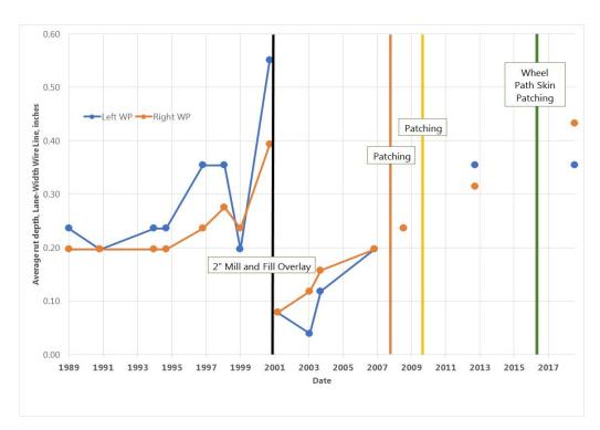
Figure 28. Time history plot of average rut depths in left and right wheel paths based on the lane width wire line edge measurement method.
