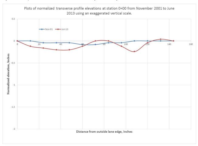
Figure 12. Exaggerated vertical scale of the normalized transverse profile at station 0+00 after the mill and fill overlay placed in October 2001.
