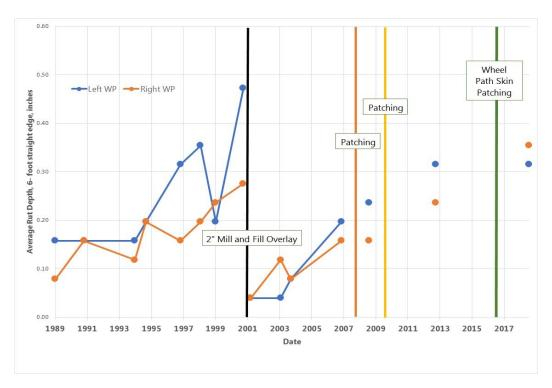
Figure 27. Time history plot of average rut depths in left and right wheel paths based on the 6-foot straight edge measurement method.
