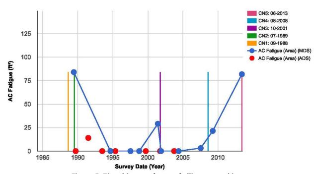
Figure 5. Time history of area of alligator cracking.
