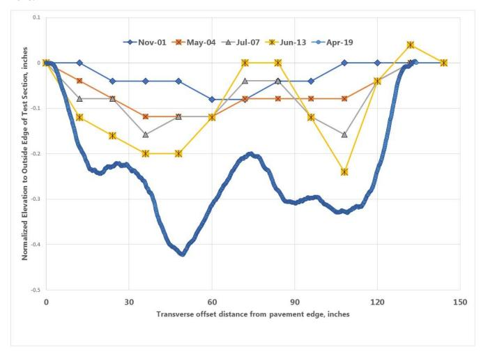
Fig 26. Comparison of historic normalized transverse profile plots at station 0+00 on section 53\_1005.
