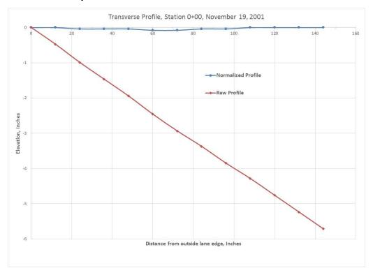
Figure 11. Normalized and raw transverse profile at stat 0+00 measured November 19, 2001, after the mill and fill overlay placed in October 2001.
