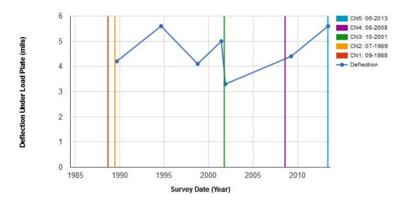
Figure 9. Time history of average deflection for the sensor located in the load plate normalized to 9,000 lb. drop load.
