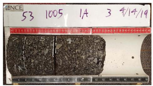
Figure 13. Image of core 1A obtained at station 200 at an offset of 0.8 feet from the outside lane edge.
