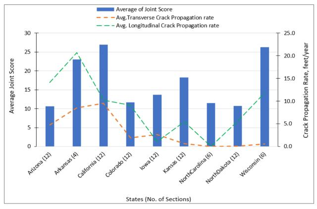
Figure 3. Relationship between Joint Score and Crack Propagation Rate for Different States
