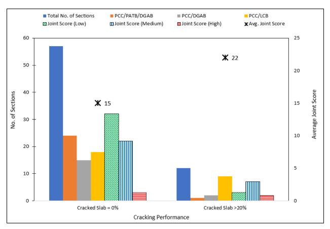
Figure 6: Effect of Base Type and Joint Score on Cracked Slabs
