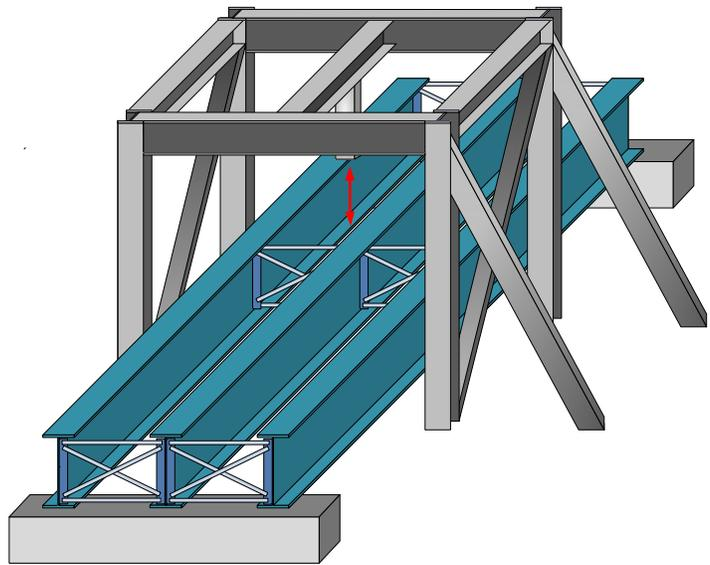
Figure 5: Test Set-up for Loading Girder System
