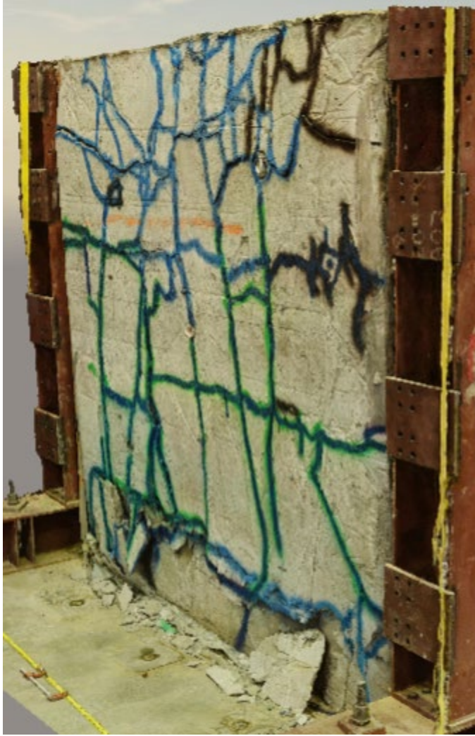
Fig. 13. Photograph of the crack pattern in the LCC on the free face opposite to the MSE wall side.
