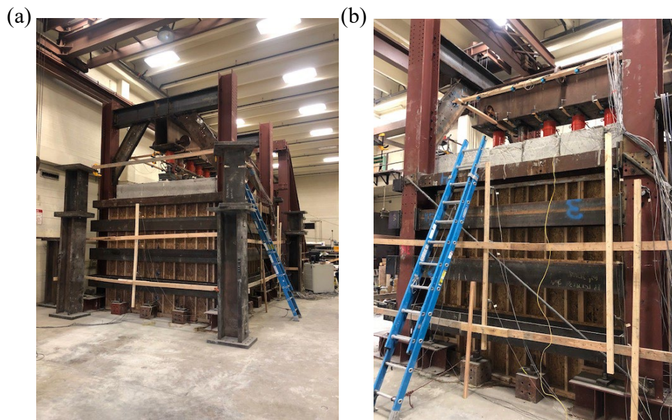
Fig. 2 Photographs showing: (a) the test box from the short side opposite from the retaining wall and (b) the test box from the long side with the concrete surcharge blocks and hydraulic jacks reacting against a longitudinal beam consisting of two deep beams.
