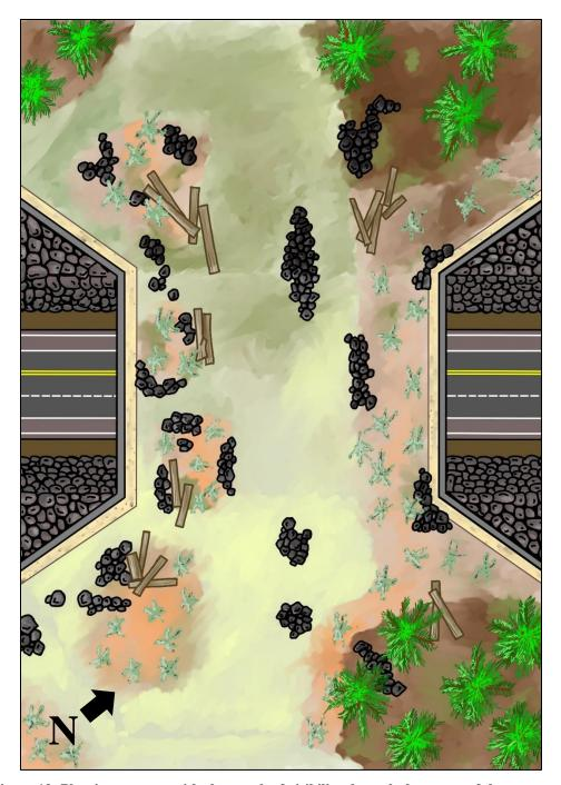
Figure 12: Planting strategy with clear path of visibility through the center of the structure.
