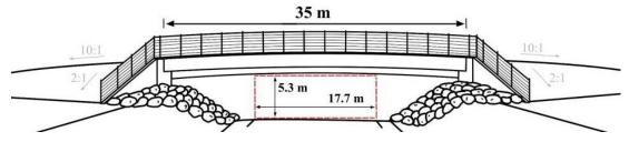
Figure 9: Elevation view of the US-97 wildlife overpass.
