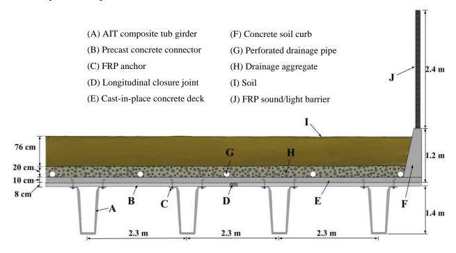
Figure 15: Cross section of the wildlife overpass showing the layout of the girders, concrete deck, soil, drainage, and barriers on the bridge span.
