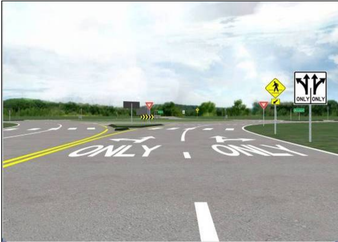
Figure 3: Example of Traditional Arrows with Words Scheme (TAW) – Type C Lane Restrictions
