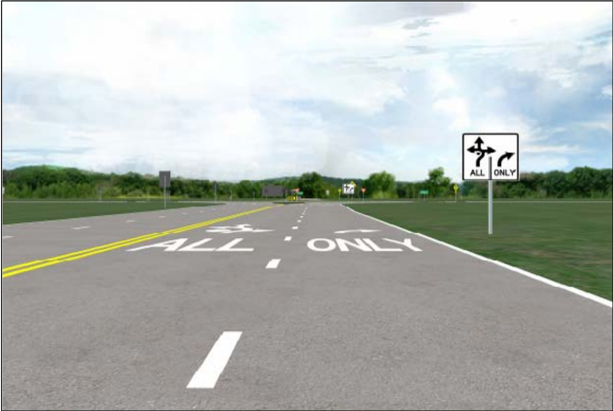
Figure 9: Example of Distal Lane Restriction Signing and Marking at 267 Feet From Yield Line
