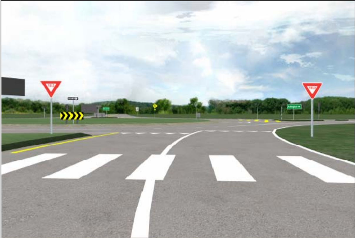
Figure 11. Yield Signs at 8 Feet From Yield Line
