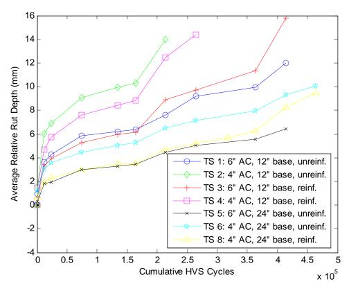
Figure 1: Rut Depths after 464k and 414k passes in Test Sections 8 and 5, respectively.
