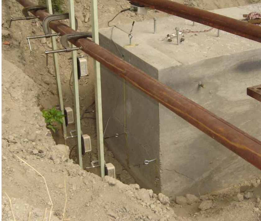
Figure 5-12 Initial cracking on the front face and side of Pile Cap 3.
