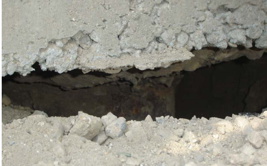
Figure 5-11 Pile Cap 2 failure in pullout.
