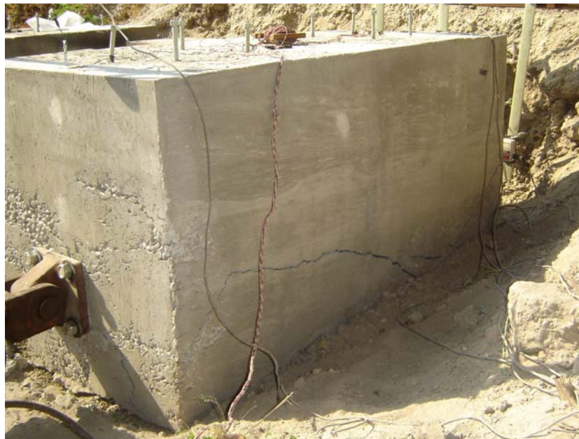
Figure 5-13 Cracking at a 90 kip load on the back and side of Pile Cap 3.
