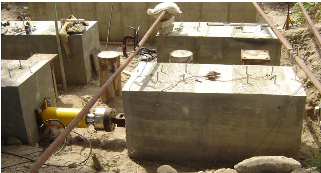
Figure 3-20 Side view of test setup prior to loading Pile Cap 3.
