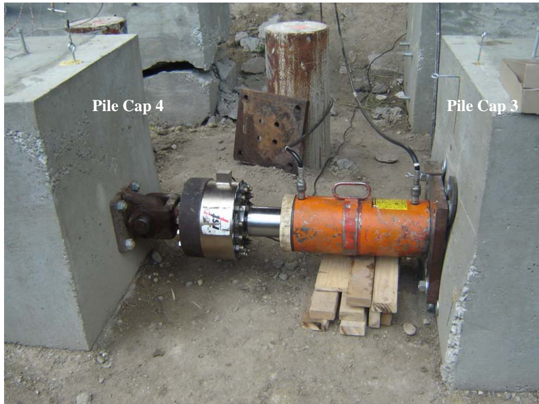
Figure 3-21 Photograph of test layout for test on Pile Cap 4.
