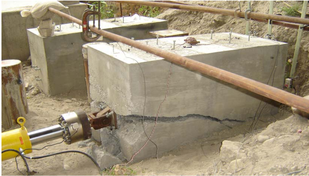
Figure 5-14 Shear crack in Pile Cap 3 at failure.
