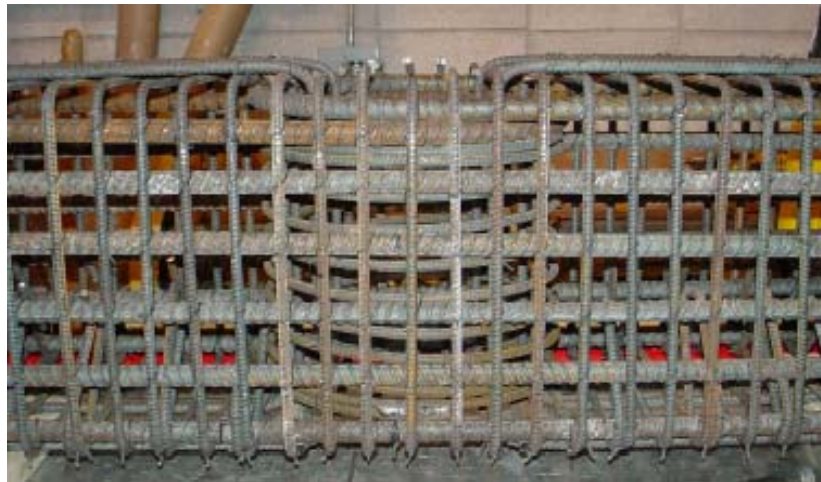
Figure 2-4 Reinforcing cage for pile cap Model 4 Montana State University (Stephens and McKittrick, 2005.
