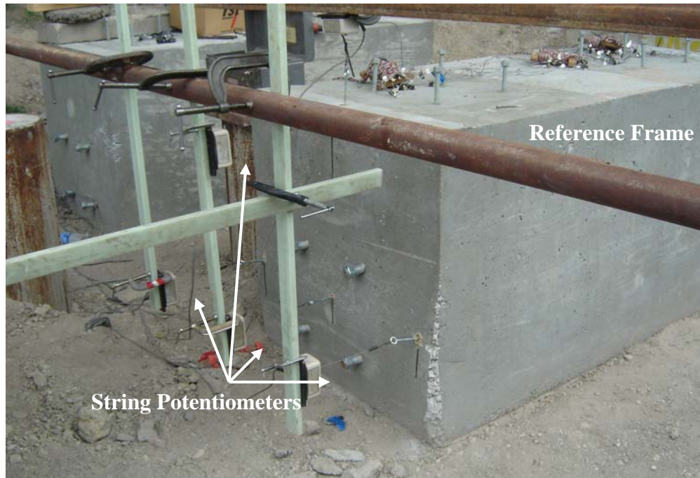
Figure 3-11 Photograph of string potentiometers setup (typical all caps).
