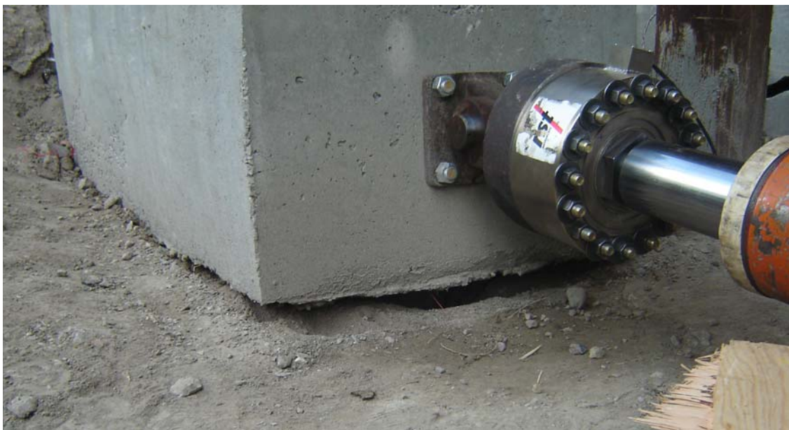
Figure 5-18 Photograph of Pile Cap 4 after pullout failure.
