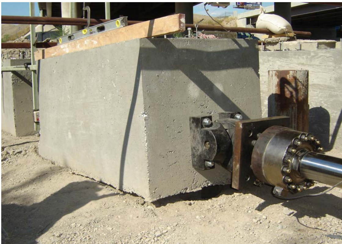
Figure 5-7 Photograph of Pile Cap 1 at failure showing uplift of the back pile.
