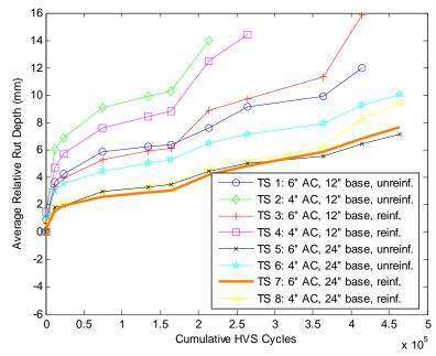
Figure 1: Average rut depth comparison of Test Section 7 after 464,000 passes and all completed test sections.
