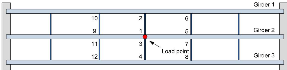
**Figure 1: Test bridge layout**
