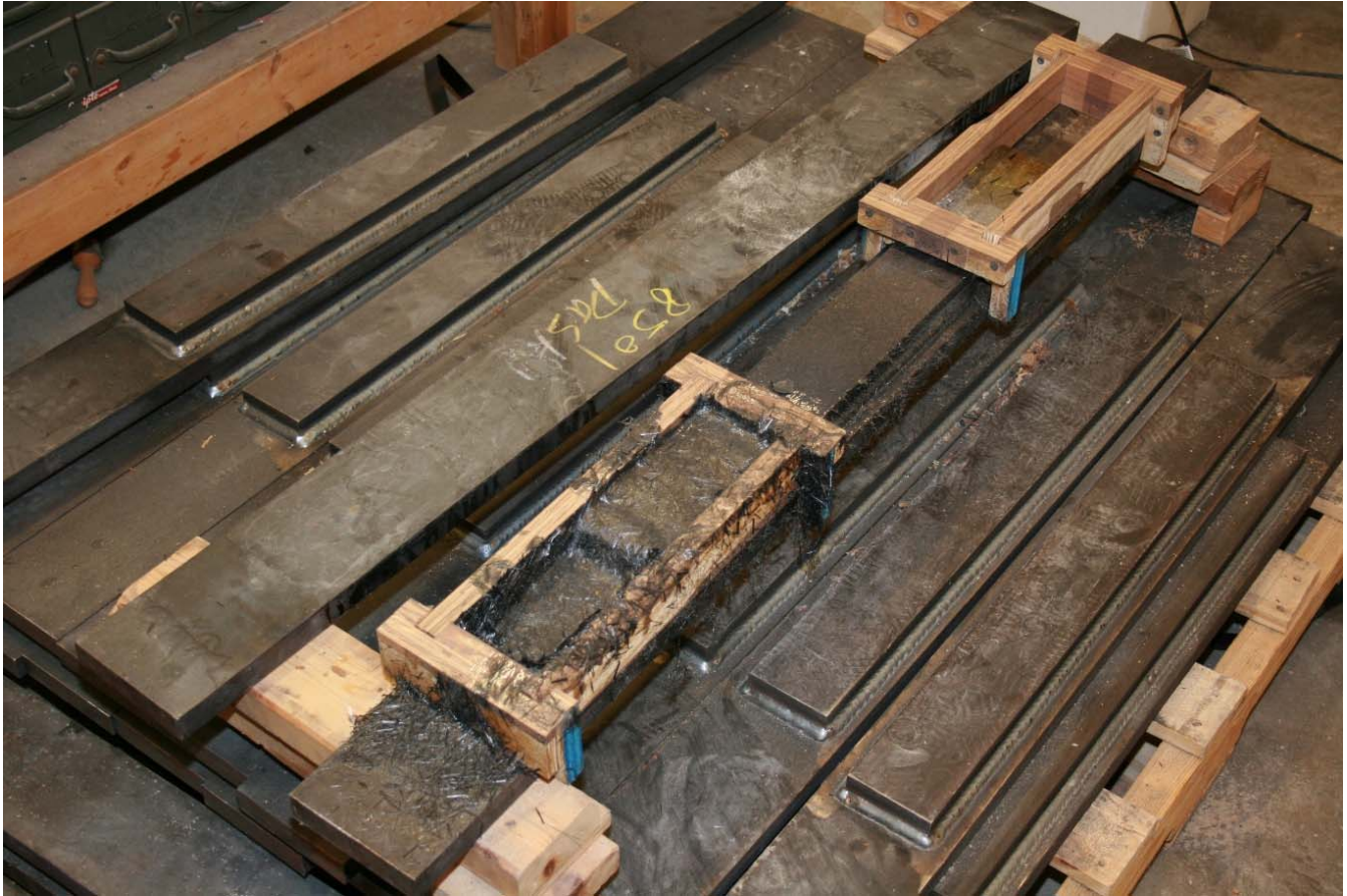
Figure 3: Chopped fiber composite sprayed on cover plate detail
