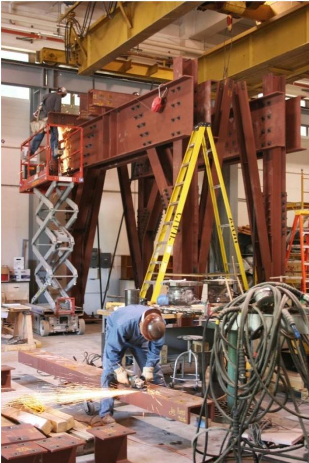
**Fig. 1. Test frame under construction**
