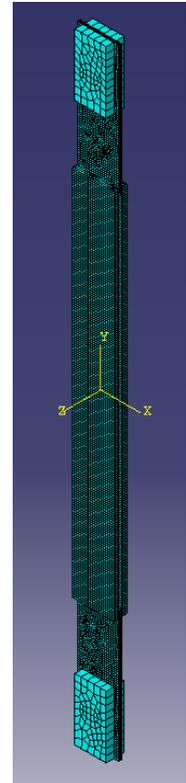
Fig. 8. Finite element model of retrofitted fatigue specimen
