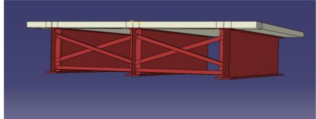
**Fig. 4.** Exposed view of lateral bracing at mid-span
