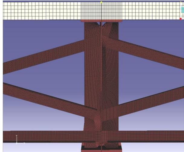
**Fig. 6.** View of internal girder with two connection stiffeners
