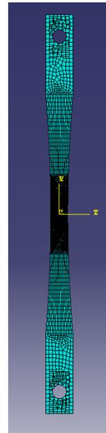
**Fig. 11.** ABAQUS model of fatigue specimen with undersized crack-stop hole
