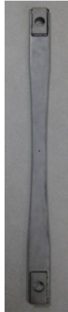
**Fig. 10.** Fatigue specimen with undersized crack-stop hole
