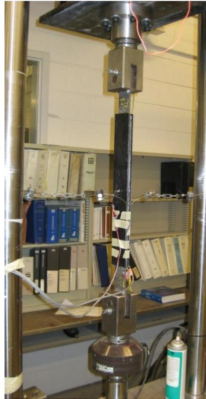
Fig. 7. Fatigue specimen with pre-existing crack, coated with chopped carbon fibers
