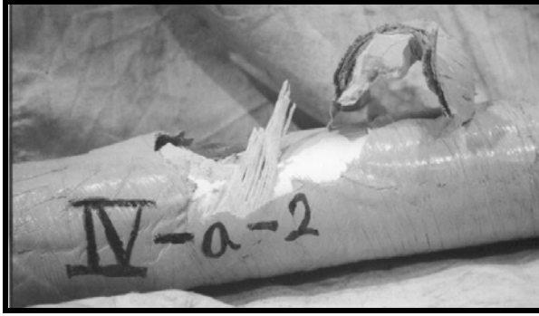
Figure 31. FRP composite failure of test IV-a (2)
