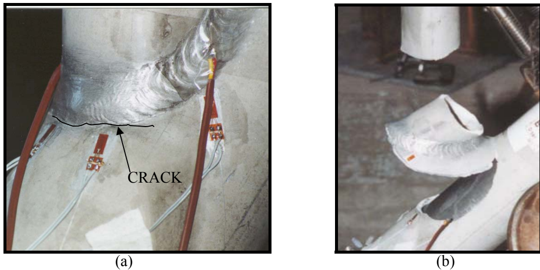
Figure 12. Fatigue test of as-is welded joint Test II-b: (a) crack prior to failure, (b) Typical failure of Series II tests
