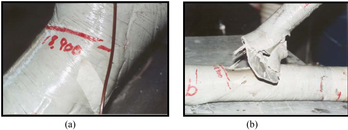
Figure 22. Test III-b: (a) Initial cracking of FRP composite, (b) Failure of Base Material, Weld, and FRP composite
