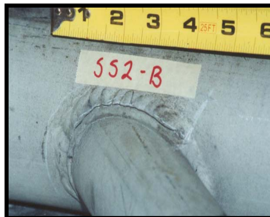
Figure 2. Crack through aluminum-welded joint of overhead sign structure
