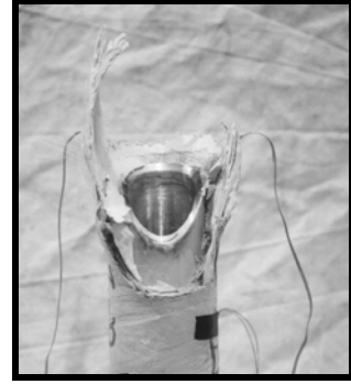
Figure 31. FRP composite failure of test IV-a (2)
