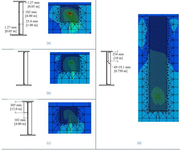
Figure 1. (a) No-retrofit stiffener. (b) Positively attached stiffener. (c) Back-up transverse stiffener. (d). Slotted connection stiffener.
