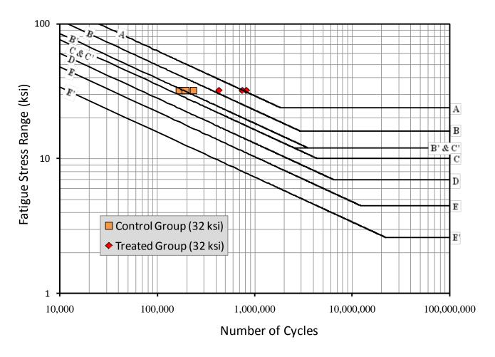
Figure 1: S-N diagram showing results for untreated and PICK-treated specimens tested at 32 ksi.
