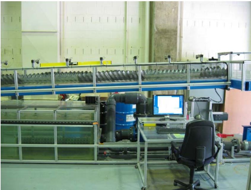
Figure 3: A series of ultra sonic flow depth meters mounted above the tilted culvert flume
