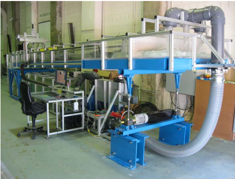
Figure 1: Finalized construction of the tilting mechanism for the culvert flume.
