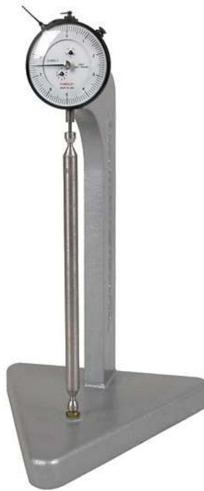
**Figure 2-3: Length Comparator [www.humboldtmg.com/c-4-p-274-id-4.html]**
