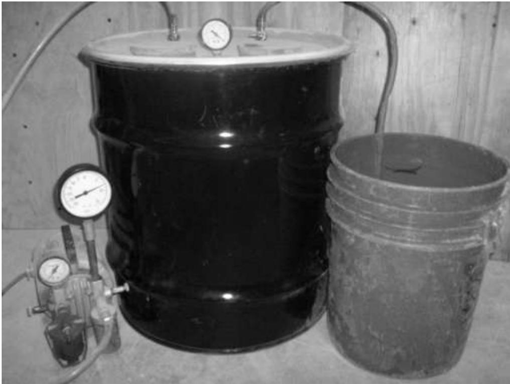
**Figure 2-4: Vacuum Saturation Equipment**
