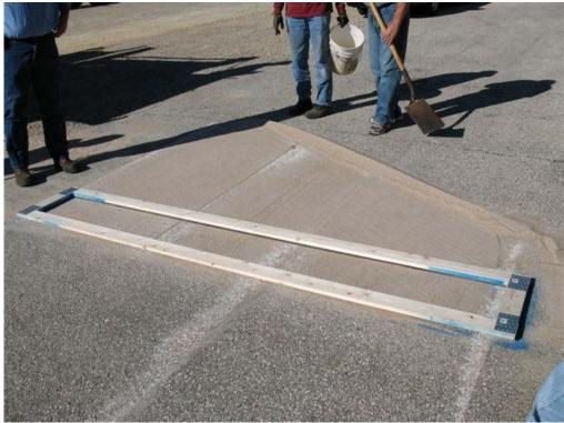
Figure 11 Frame used to contain sandblast sand
