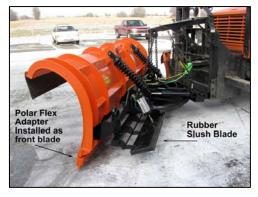
Air lines were run to the front of the truck to control the squeegee, and Iowa DOT installed electronic switches and relay valves. Consideration was given to how high to mount the plow and placement of the holes to attach it.
