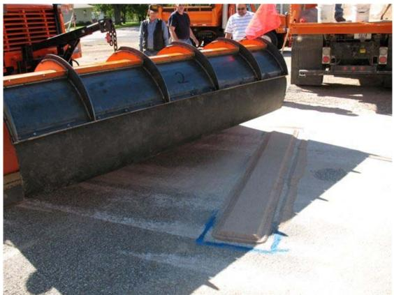
Figure 3 Plow with Active Adapter system
