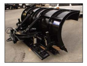
The Henke Manufacturing prototype featured a custom-built flexible cutting edge, an Olofsfors scarifying blade and a squeegee blade.
