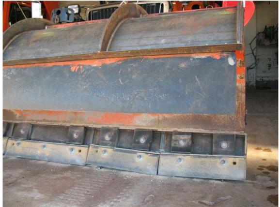
Figure 2 Flexible Edge with rebar under blade to show the blades ability to adjust to roadway contours
