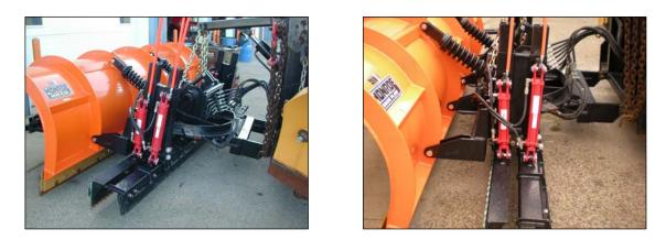
Three blades are used on Monroe Truck Equipment's prototype: the ABAS flexible blade system, an Olofsfors scarifying blade and a squeegee blade.
