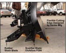
The prototype plow was mounted to a 2007 International multipurpose dump truck. Approximate total weight of the prototype plow is 2,750 lbs.
