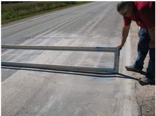
Figure 20 Profile of roadway to show wheel rut
