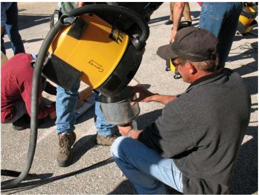
Figure 19 Capturing sand for weighing
