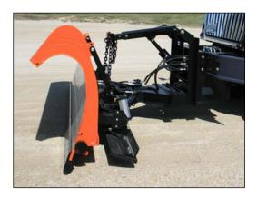
The prototype developed by Henderson Products Inc. included two blades: a PolarFlex cutting blade and rubber squeegee blade.
