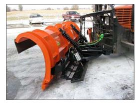
Flink Company's two-blade prototype included a PolarFlex flexible cutting edge and a rubber squeegee blade.
