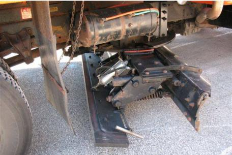
Figure 9 Standard Iowa DOT underbody plow with squeegee blade
