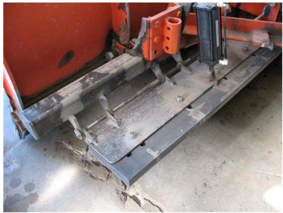
Figure 4 Squeegee blade attached to plow frame behind Active Adaptor System
