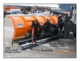
The prototype plow was installed on an International 7600 tri-axle dump truck. The multiple-blade setup added about 500 lbs. to the typical Monroe plow, for a total weight of approximately 3,200 lbs.
