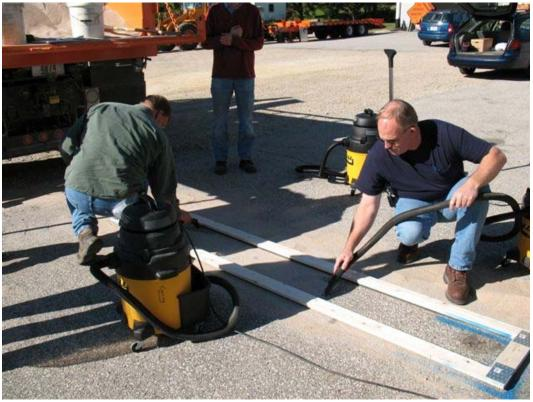
Figure 18 Collecting sand from frame after plow pass
