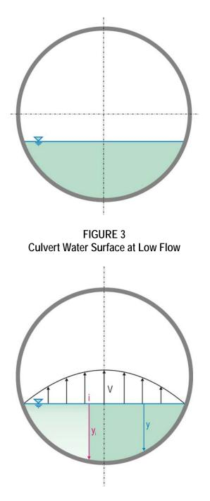
FIGURE 4 Determine Flow Depth and Velocity Distribution from Lab and CFD Tests
