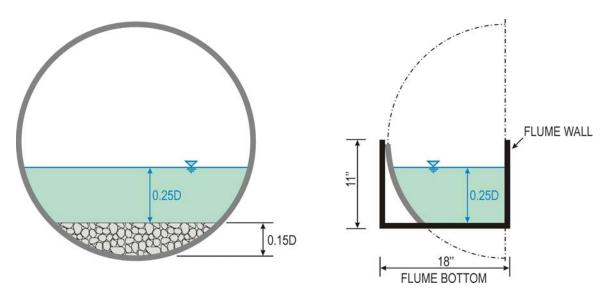
FIGURE 8 Bed Elevation at 0.15 culvert diameter and symmetrical half of Flume Culvert Model
