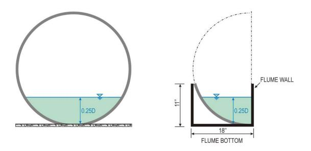
FIGURE 7 Bed Elevation at 0 culvert diameter and symmetrical half of Flume Culvert Model
