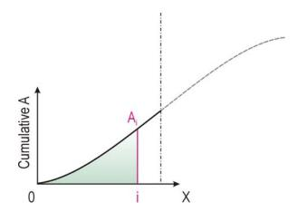
FIGURE 5 Determine the Cumulative Area from the Wall to the Centerline
