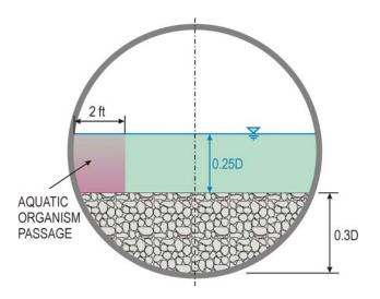
FIGURE 12 Bed Elevation at 0.30 culvert diameter and 2 ft AOP for CFD Tests
