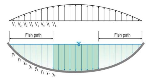
FIGURE 2 Computation of the Dimensions of the Flow Path for the Selected Fish Design Criteria of Velocity and Depth
