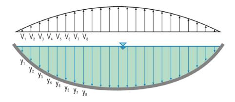
FIGURE 1 Variation of Flow Velocity and Depth in a Cross-Section of a Corrugated Metal Pipe
