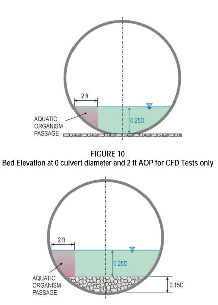
FIGURE 11 Bed Elevation at 0.15 culvert diameter and 2 ft AOP for CFD Tests
