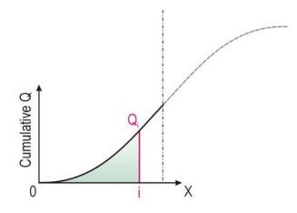
FIGURE 6 Determine the Cumulative Discharge from the Wall to the Centerline Use equation 1 to determine the average velocity:
