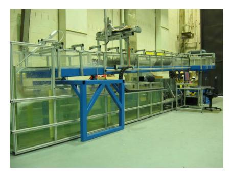
FIGURE 13: Fish Passage Culvert Flume
