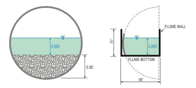
FIGURE 9 Bed Elevation at 0.30 culvert diameter and symmetrical half of Flume Culvert Model
