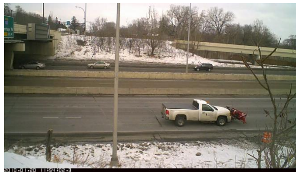
Class 3 pickup truck classified as a SU Truck by the GTT Canoga Microloops because of the plow mounted on the front of the truck.
