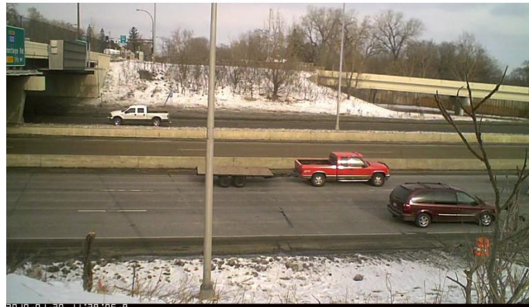
Pickup truck in Lane 3 hauling a trailer that was detected as a large truck.
