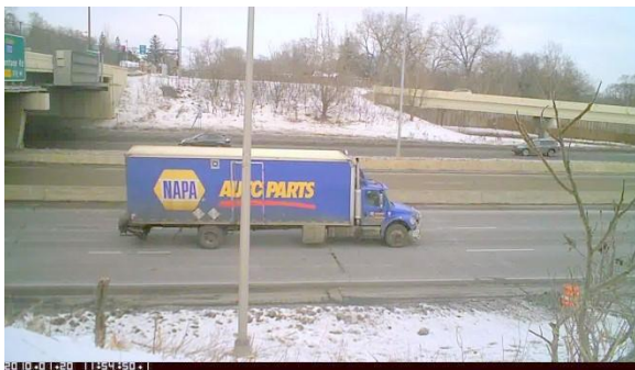
Long Class 5 truck classified as a MU Truck by the GTT Canoga Microloops.
