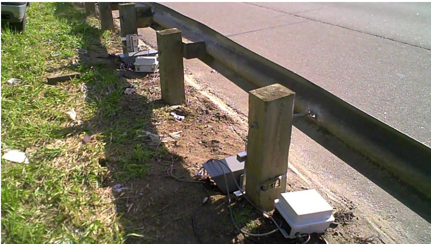
Two AxleLight sensors set up in a speed trap configuration.
