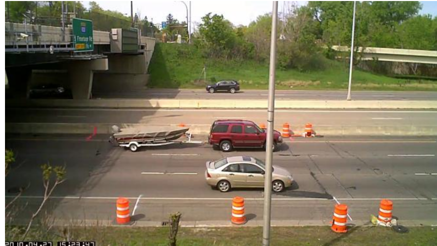
35.3-foot SUV pulling trailer measured at 17 feet long by Canoga Microloops.
