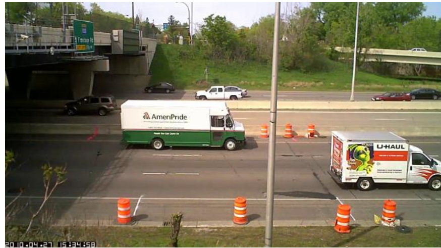
25.1 foot truck measured at 14 feet long by Canoga Microloops
