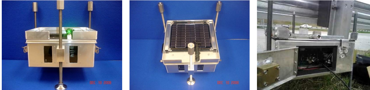
Figure 27. TIRTL with Portable Enclosure
