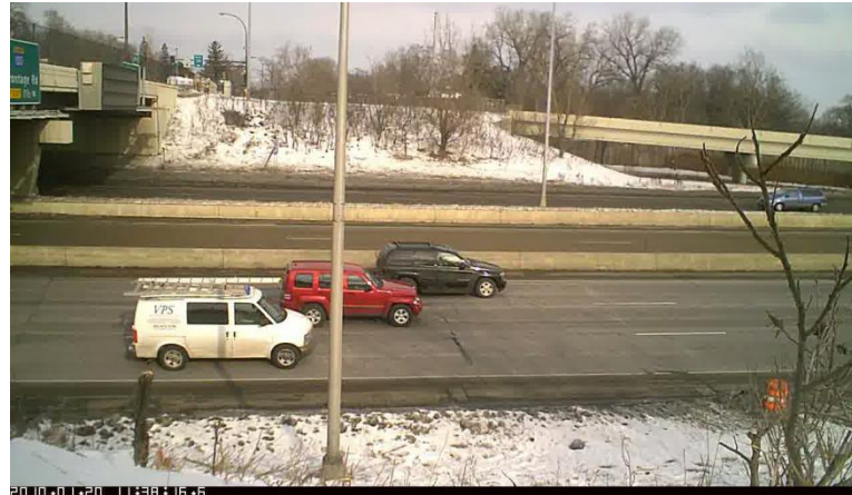
SUV in Lane 3 (far lane) detected as a 24-foot vehicle.
