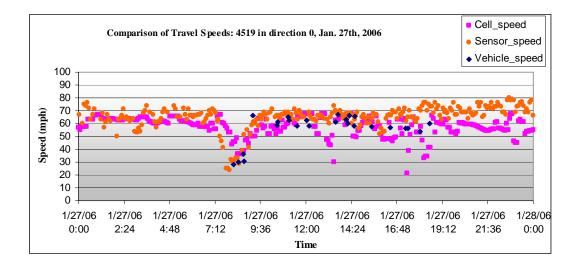
Figure 6-2 Comparison of travel speeds: I-695 outer loop @ US 40 West, 27 January 2006
