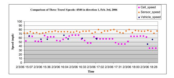
Figure 6-53 Comparison of Three Travel Speeds: I-695 Inner Loop @ I-95, 3 February 20
