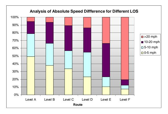
Figure 4-12 Absolute speed difference for different LOS
