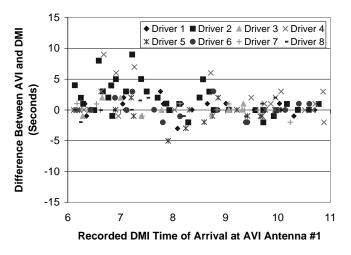
FIGURE 6 Difference between AVI and test vehicle (DMI) traveltime estimates by driver for entire corridor.
