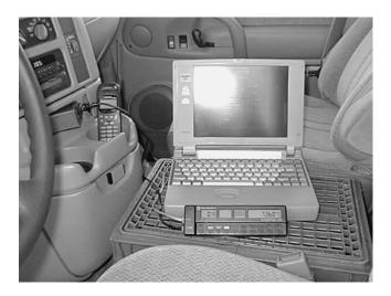
FIGURE 5 DMI instrumentation in test vehicle.
