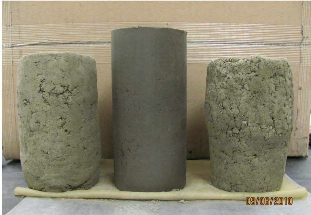
Figure 8.15 Deformed Soil Samples at High Moisture Content
