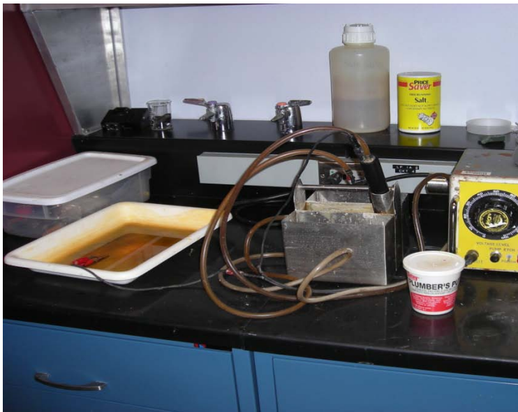
Fig 20. Electropolishing set-up; specimen preparation for X-ray diffraction
