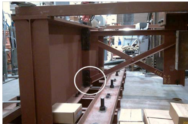
Fig 5. View of 9-ft girder test set-up; bottom web gap (representative of real top web gap) is circled.
