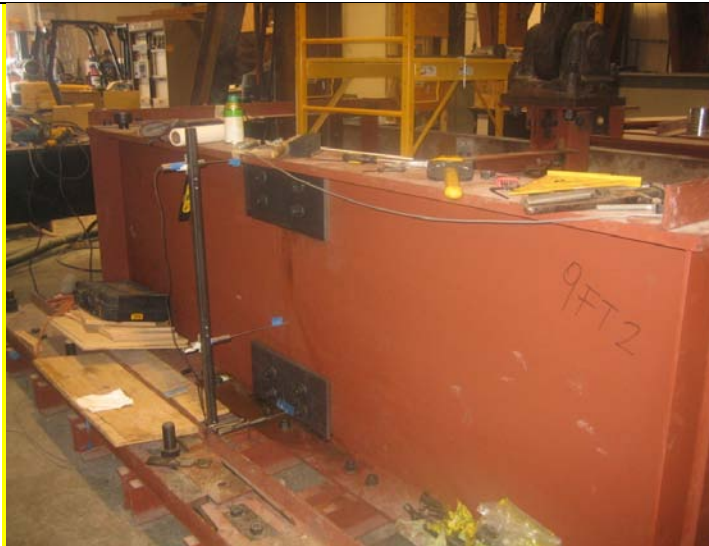
Fig 9. Fascia view of girder after angle retrofit has been applied in both the top and bottom web gaps.
