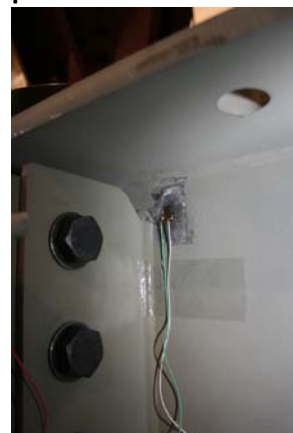
Fig 3. View of web gap region in test section with applied strain gage
