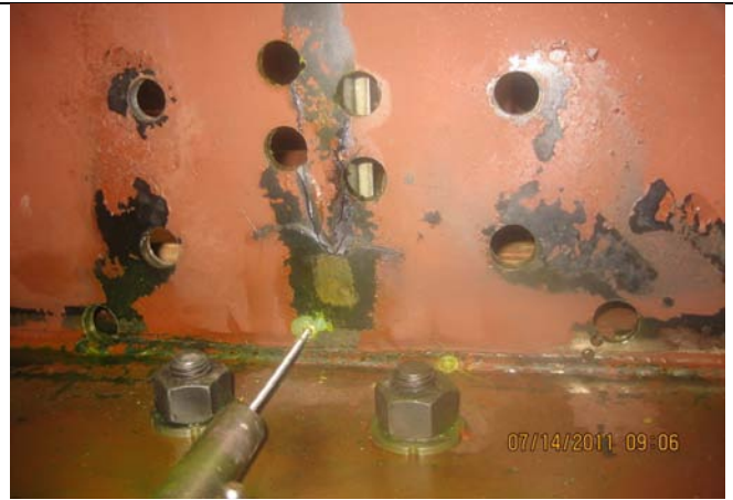
Fig 17. Specimen 2 with drilled crack-stop holes (six) in bottom web gap region
