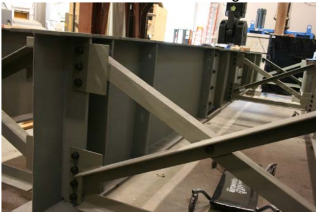
Fig 2. Alternate view of three-girder test set-up and end cross-frame
