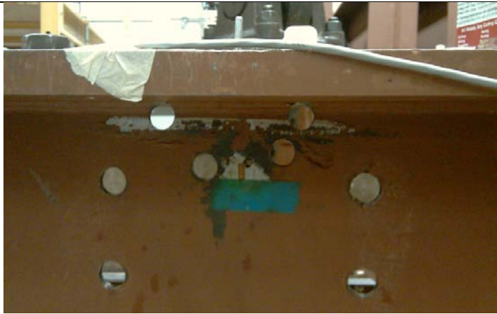
Fig 16. Specimen 2 with drilled crack-stop holes (four) in top web gap region
